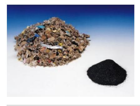
Figure 4 CARBOR: solid fuel produced from waste.
