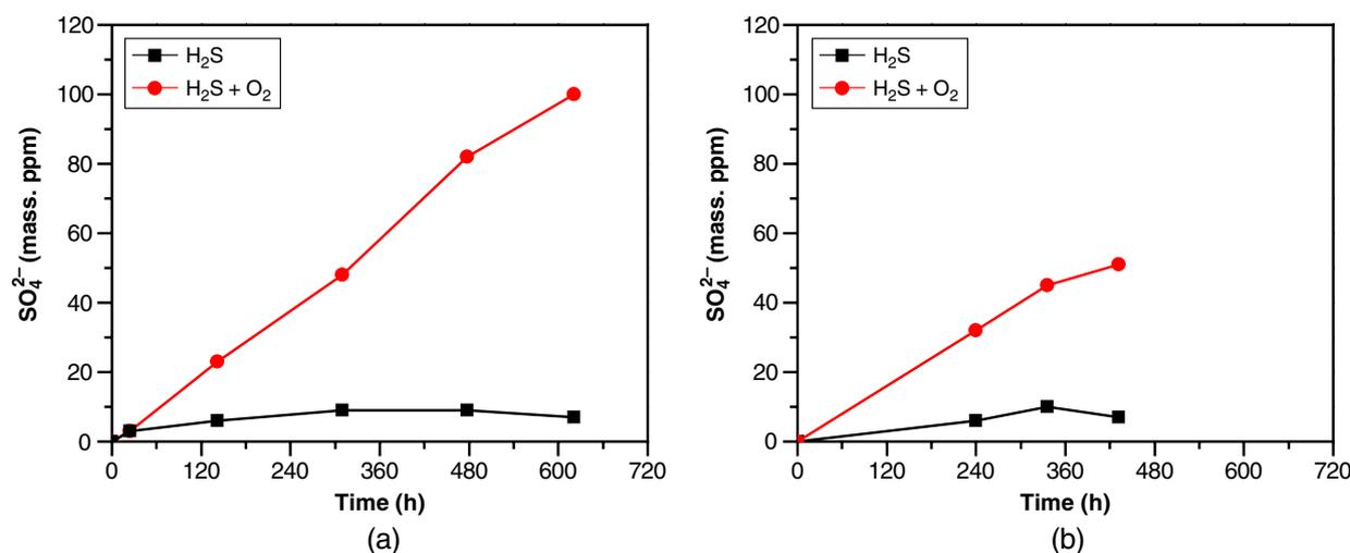
**FIGURE 2.** Time evolution of sulfate concentration for the tests at 100 kPa and 10 kPa H<sub>2</sub>S in model systems.
