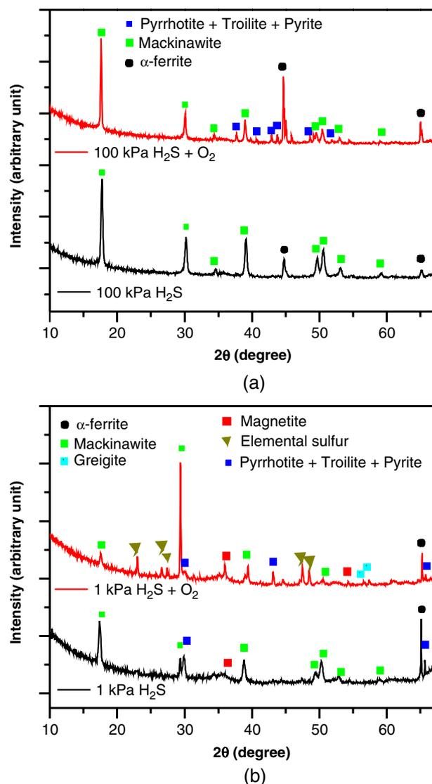
**FIGURE 3.** XRD patterns from pure iron surfaces after long-term exposure to H<sub>2</sub>S-containing 35 g/L NaCl (24°C), with and without 500 ppb oxygen contamination, at (a) P<sub>H<sub>2</sub>S</sub> = 100 kPa and (b) 1 kPa.
