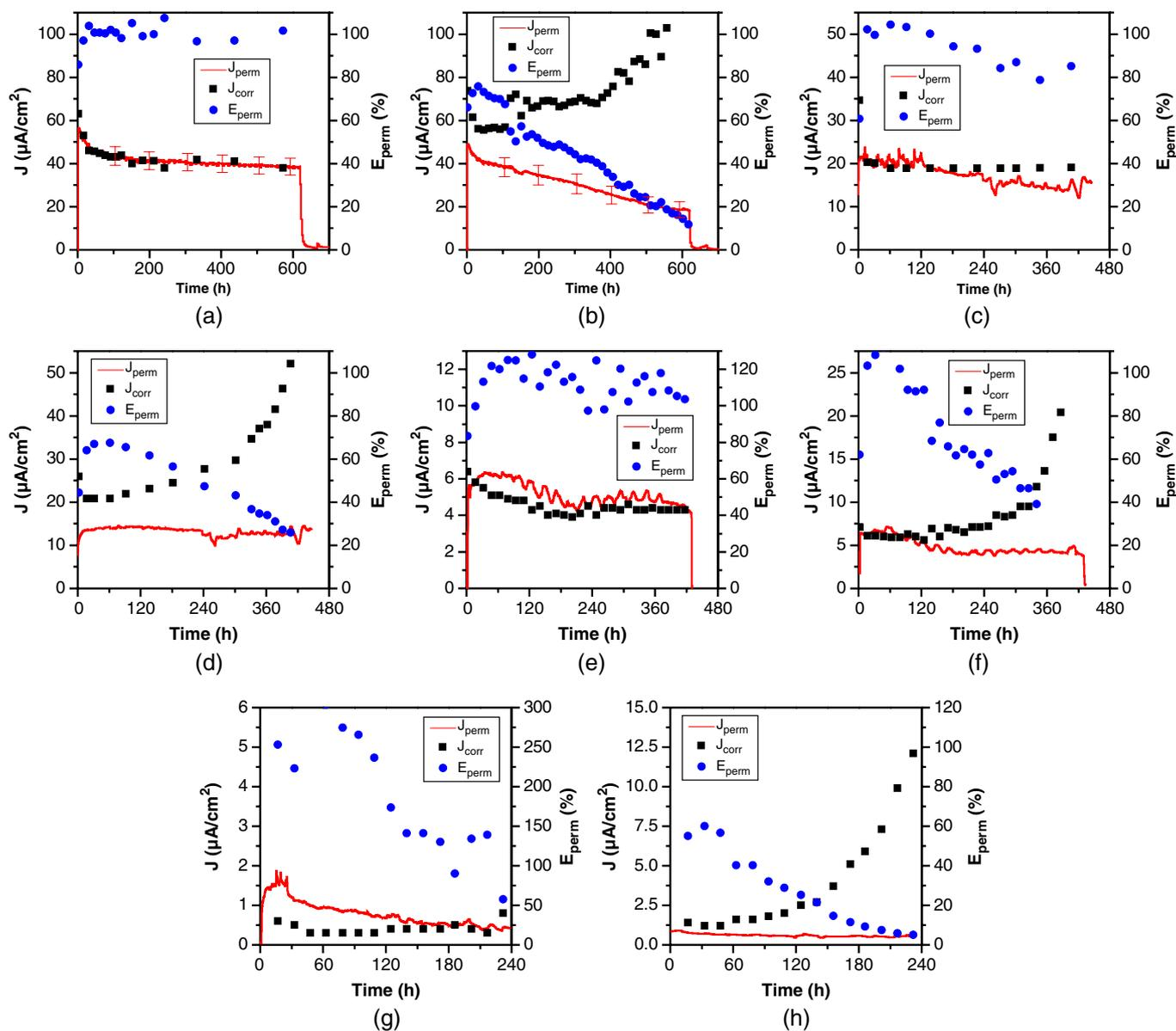
**FIGURE 7.** Comparisons between  $J_{\text{corr}}$  and  $J_{\text{perm}}$ , and evolution of the permeation efficiency, as a function of time. Tests at (a, b) 100 kPa, (c, d) 10 kPa, (e, f) 1 kPa, and (g, h) 0.1 kPa, (a, c, e, g) without and (b, d, f, h) with  $\text{O}_2$  contamination.
