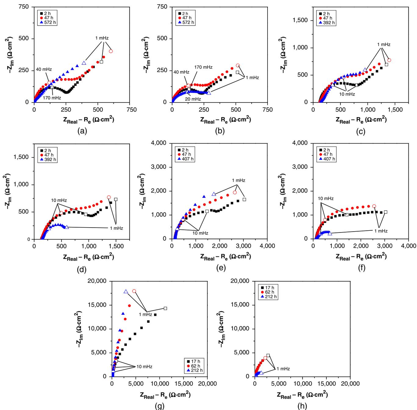
**FIGURE 4.** Typical impedance of pure iron in 35 g/L NaCl solution saturated with  $H_2S$  at (a, b) 100 kPa, (c, d) 10 kPa, (e, f) 1 kPa, and (g, h) 0.1 kPa; (a, c, e, g) without and (b, d, f, h) with  $O_2$  contamination.
