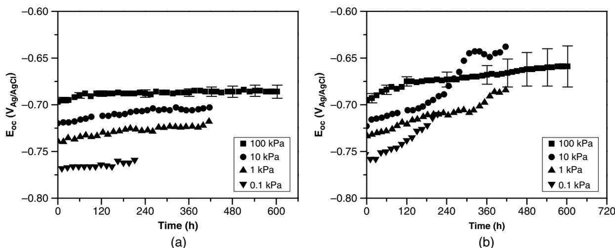
**FIGURE 6.** Time evolution of open-circuit potentials of pure iron exposed to 35 g/L NaCl solution saturated with  $H_2S$  at various partial pressures for 2 to 4 weeks, (a) without oxygen and (b) with oxygen contamination.
