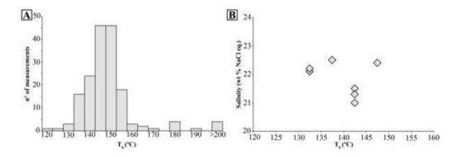
**Figure 7.** Homogenization temperatures  $(T_h)$  and salinity data of aqueous and presumably primary fluid inclusions in nodular and tabular calcite obtained from the Arab Formation. (A) Histogram for all measured aqueous and presumably primary fluid inclusions. Most  $T_h$  values range between 135 and 155°C. (B) Cross-plot showing that there is no correlation between  $T_h$  and salinity.
