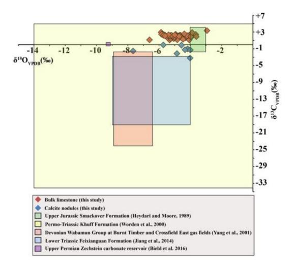
Figure 6. Carbon *versus* oxygen isotope cross plot showing that nodular calcite has lower  $\delta^{13}C_{VPDB}$  values than the bulk limestone samples from the Arab Formation. Isotope compositions of calcite associated with TSR from other studies are included for purpose of comparison. The calcites in this study have slightly depleted  $\delta^{13}C_{VPDB}$  values compared to bulk limestone samples.
