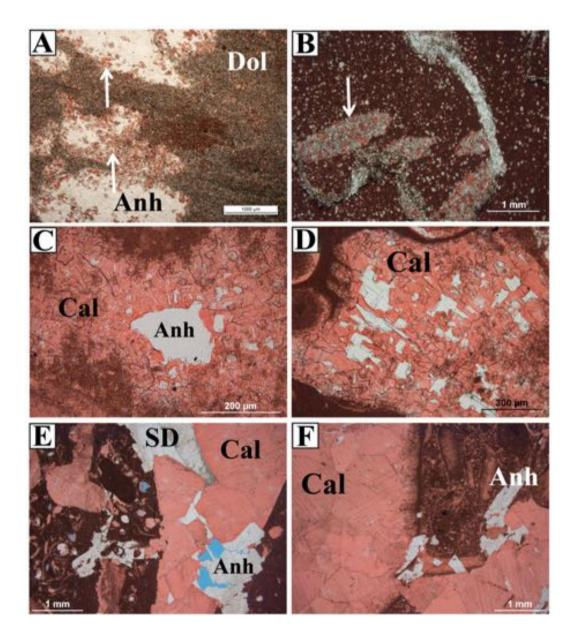
**Figure 4.** Photomicrographs (PPL) of calcite (Cal; stained red by alizarin red) in close relationship with anhydrite on the crest of the anticline. (A) Calcite concentrated mainly along the edges of the anhydrite nodules (arrow) in a partly dolomitized mudstone (outer ramp facies). (B) Partly dolomitized calcite crystals in the lagoon facies. (C) and (D) Calcite
