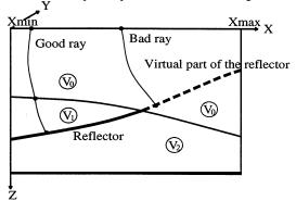
Fig. 1 Example of a model presenting a pinch-out. Continuous lines are the reflecting parts of interfaces, the dashed line is a virtual part that has no physical meaning. Specifying a ray signature allows to sort good and bad rays.
