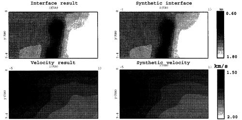
Fig. 6 Comparison between the synthetic model and the model obtained by reflection tomography for the tertiary layer. The RMS misfit is 0.2ms, the maximum misfit is 39.7ms (only 2 misfit values over 120390 are greater than 10ms).
