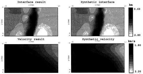
Fig. 7 Comparison between the synthetic model and the model obtained by reflection tomography for the chalk layer. The RMS misfit is 0.7ms, the maximum misfit is 77.8ms (only 45 misfit values over 129300 are greater than 10ms).
