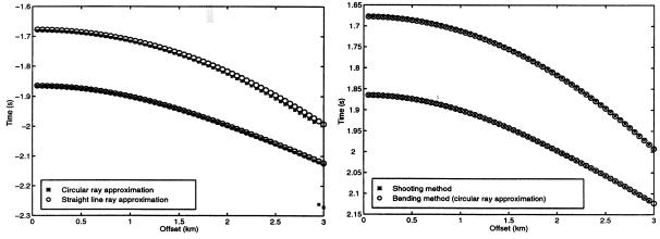
Fig, 5 Triplicated multi-offset times associated with the chalk base of the synthetic model for a CMP (x = 6775m) y = 4125m). Left side: comparison between our bending method with the circular ray approximation and a bending method with a straight line ray approximation. Right side: comparison between our bending method with the circular ray approximation and a shooting method (Clarke et al., 1994). Two initialization angles for the bending provide the two branches.
