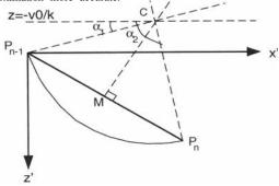
Fig. 2 Description of the traveltime calculation for circular ray path. C is the center of the circle,  $P_{n-1}$  and  $P_n$  are successive impact points.  $v_0$  is the mean of the velocity values at  $P_{n-1}$ ,  $P_n$ ,  $M \cdot k$  is the vertical velocity gradient.
