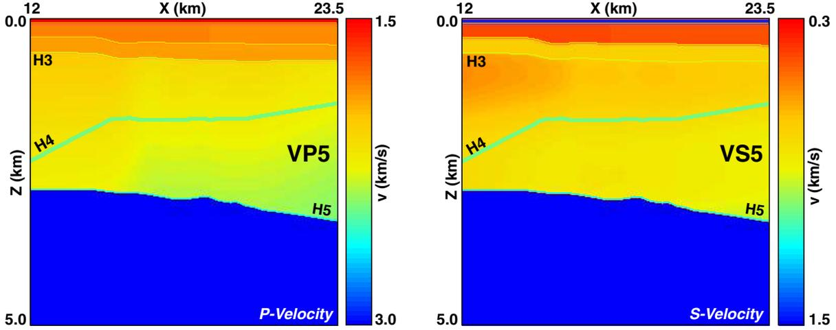
Figure 11: Solution model 3 obtained by tomography with a constrain on  $\delta$  parameter to remain positive. The RMS value of the traveltimes misfits is  $6.371ms$ . The anisotropy parameters values are:  $\eta = 6.2\%$  and  $\delta = 2\%$ .
