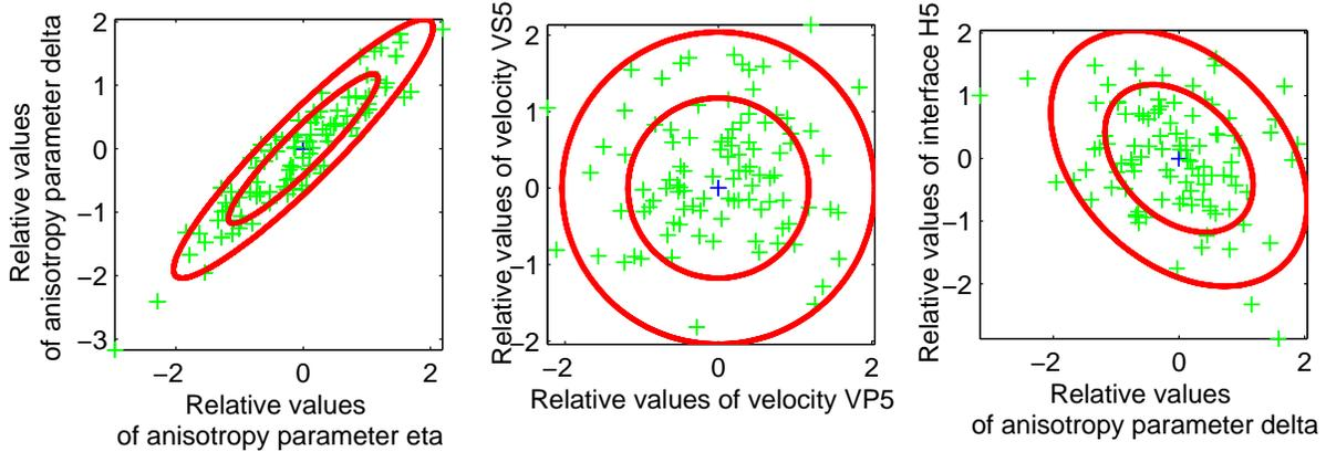
Figure 9: 68% and 95% isovalues of the marginal probability density function for the anisotropy parameters  $\eta$  and  $\delta$  (left), P-velocity and S-velocity (middle),  $\delta$  and the interface depth of reflector h5 (right). The represented values are the relative ones (for instance:  $\frac{\eta - \eta^{sol}}{|\sigma_\eta|}$ , where  $\sigma_\eta$  is the standard deviation for the anisotropy parameter  $\eta$ ). The crosses represent the MP values of the 100 simulated models.
