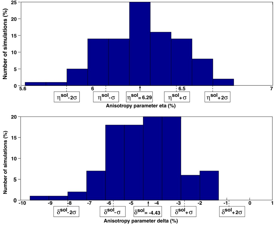
Figure 8: Histograms of the 100 simulated velocity models. Top: anisotropy parameter  $\eta$ . Bottom: anisotropy parameter  $\delta$ .  $\sigma$  corresponds to the standard deviation on the anisotropy parameter  $\eta$  ( resp.  $\delta$ ) given by the macro-parameter method.(see section 4.2).
