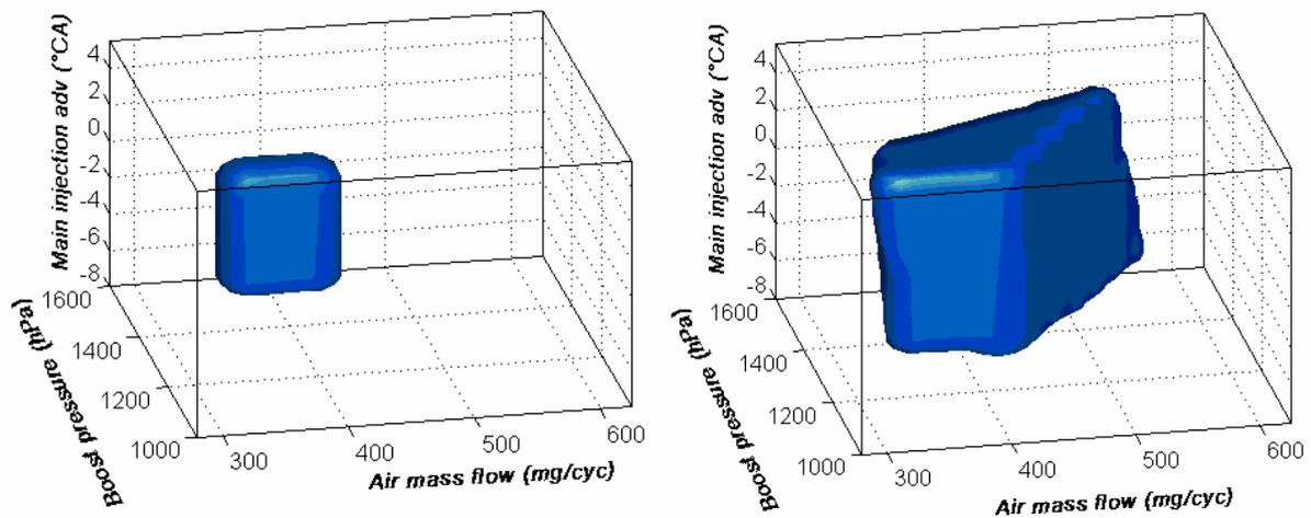
Figure 8: comparison of local hypercubic domain (left) and enlarged OS (right)
