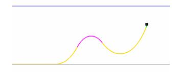
Figure 1: initial cable geometry. The pink part of the curve represents the cable with buoyancy modules.
