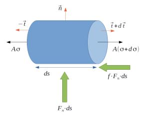
Figure 4: mechanical equilibrium on an elementary wire part.
