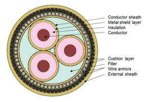
Figure 2: typical cross section of MVAC cable.
