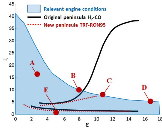
Fig. 12: Detonation peninsula calculated for TRF-air mixtures ( $P_0 = 50$  bar,  $T_0 = 1100$  K,  $\phi = 1$ , no dilution).
