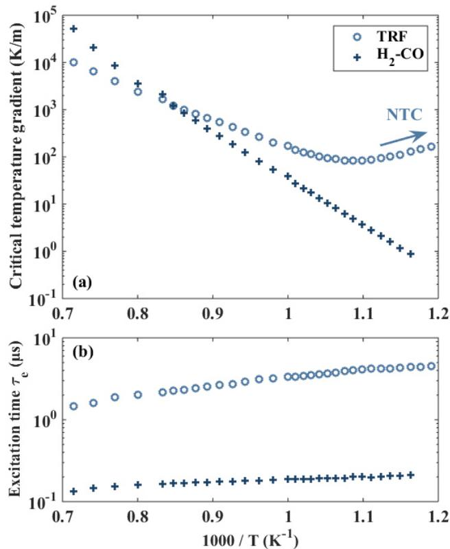
Fig. 1: Critical temperature gradients (a) and excitation times (b) computed for 50% $H_2$ -50% $CO$ -air and TRF-air mixtures at 50 bar (stoichiometric conditions, no dilution).
