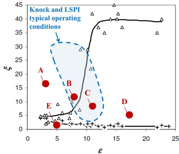
Fig. 5: Position of analyzed conditions in the original detonation peninsula [4].
