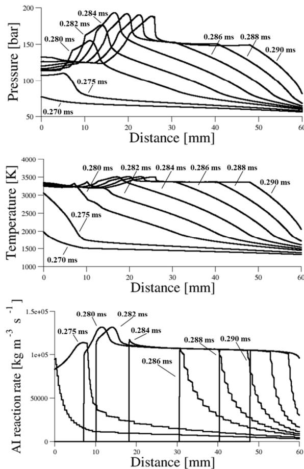
Fig. 10: Hot spot auto-ignition for case E ( $r_0 = 8.7$  mm,  $\Delta T_0 = 4.7$  K,  $\varepsilon = 5$ ,  $\xi = 1$ ,  $P_0 = 50$  bar,  $T_0 = 1100$  K,  $\phi = 1$ ,  $\tau_i = 0.286$  ms). Time sequence from 0.270 ms up to 0.290 ms.
