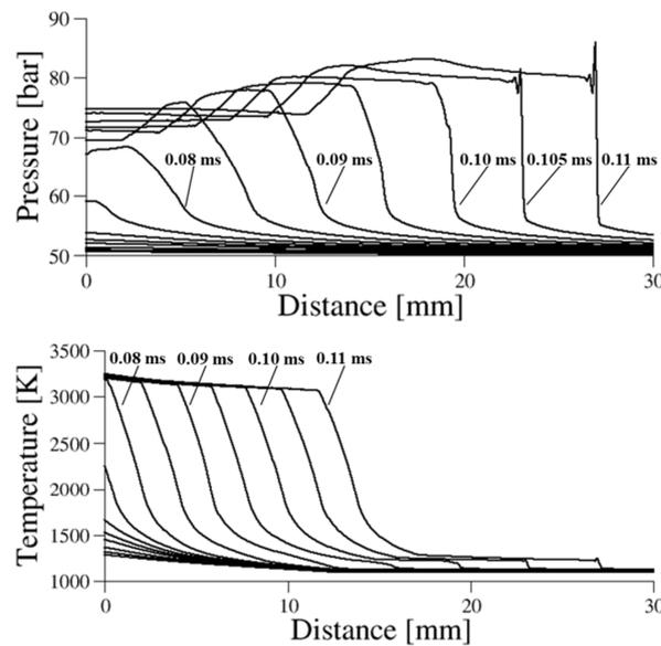
Fig. 7: Hot spot auto-ignition for case B ( $r_0 = 12.2$  mm,  $\Delta T_0 = 131.8$  K,  $\varepsilon = 7.9$ ,  $\xi = 10.7$ ,  $P_0 = 50$  bar,  $T_0 = 1100$  K,  $\phi = 1$ ,  $\tau_i = 0.286$  ms). Time sequence from 0.03 ms up to 0.11 ms.
