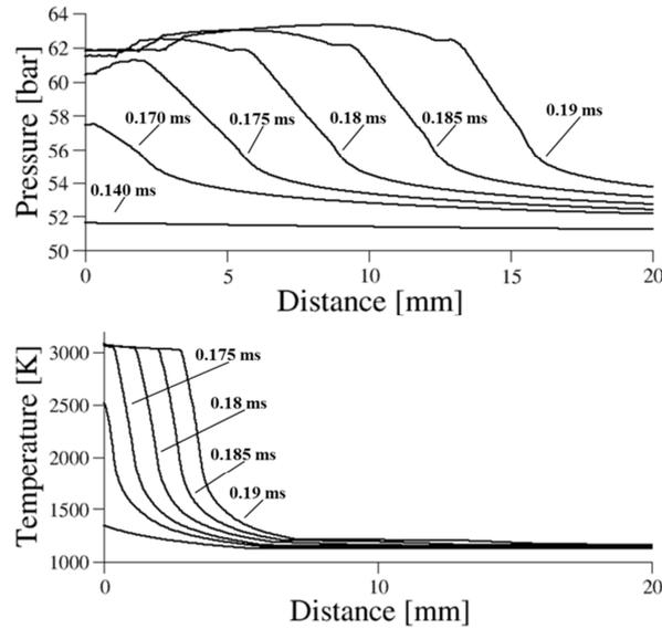
Fig. 6: Hot spot auto-ignition for case A ( $r_0 = 5.2$  mm,  $\Delta T_0 = 56.2$  K,  $\varepsilon = 3.1$ ,  $\xi = 16$ ,  $P_0 = 50$  bar,  $T_0 = 1100$  K,  $\phi = 1$ ,  $\tau_i = 0.286$  ms). Time sequence from 0.14 ms up to 0.190 ms.
