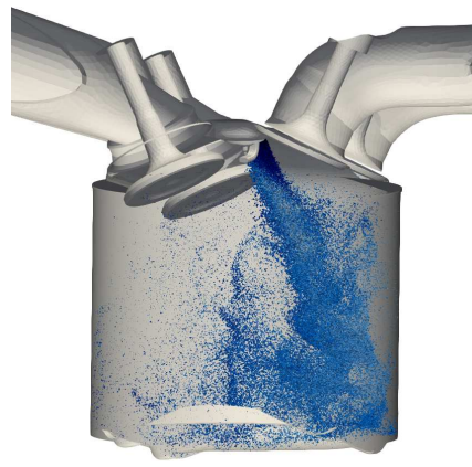
Figure 7. Image of injected droplets in the cylinder during intake valve opening for one LES cycle. Droplets are colored by their temperature.
