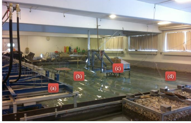
Fig. 10. Experimental setup at AAU. The waves are generated by the wave generation system (a) and the wave elevation is measured by a series of wave gauges (b). The waves then reach the WEC model, where the wave energy absorption takes place (c). Finally, they reach the beach where the termination takes place by a scattering process (d).
