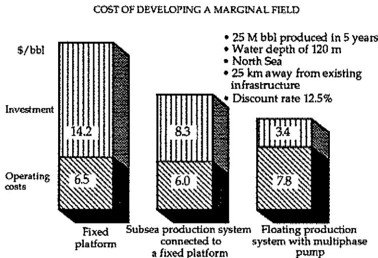
Lastly, new concepts combining subsea well heads with floating light production systems connected by flexible pipelines are making possible the economic development of marginal fields located in mature zones such as the Gulf of Mexico or the North Sea.
