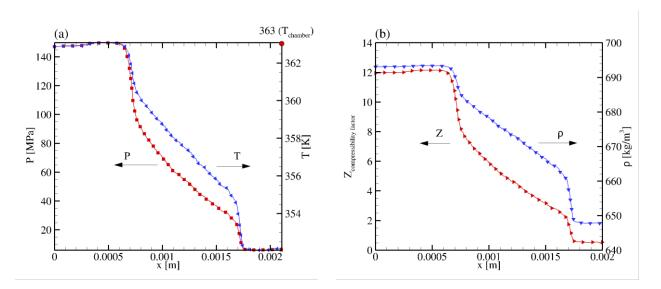
Figure 17 (a) In-nozzle evolution of pressure and temperature from the sac to the chamber. (b) In-nozzle 13 evolution of compressibility factor and density from the sac to the chamber. 14
