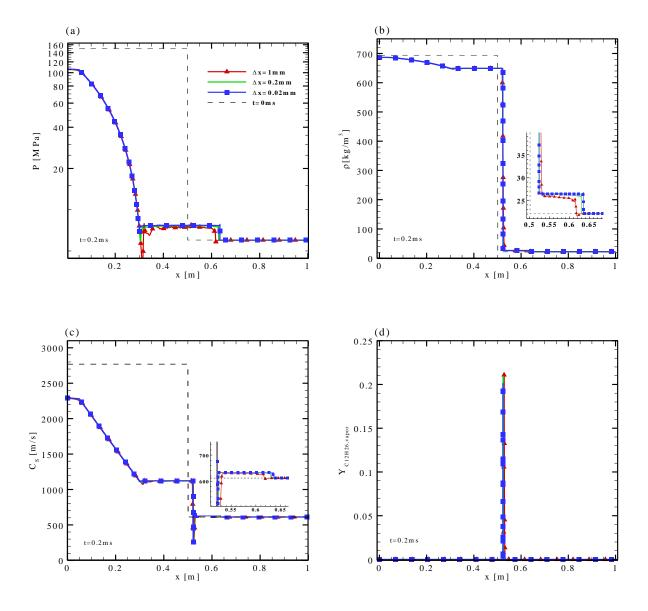
Figure 6 1D two-phase shock tube operated with Spray A conditions ( $P_{inj.} = 150 MPa, T_{fuel} = 363 K, P_{amb.} = 6 MPa, T_{amb.} = 900 K$ ) using the 4EQ-PR-EQ model. (a, b, c, d) denotes the evolution of pressure, density, speed of sound and mass fraction of vaporous dodecane at an instant of 0.2 ms with a varied mesh resolution from 1 mm, 0.2 mm to 0.02 mm and a CFL value equaling 0.2.
