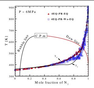
Figure 13 T-<sub>x</sub> diagram of n-C<sub>12</sub>H<sub>26</sub> and N<sub>2</sub> system at a pressure of 60 bar.  $T_E$  denotes the equilibrium temperature between the mixture.  $T_F$  symbols the frozen temperature or adiabatic mixing temperature. The red scattered triangles are obtained from CFD modelling with 4EQ-PR-EQ model at t = 50 µs. The blue scattered squares are obtained from CFD modelling with 4EQ-PR-Wo-EQ model at t = 50 µs.
