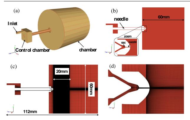
1 Figure 7 (a) Configuration of whole computational zone, note the lower control chamber below the fuel
