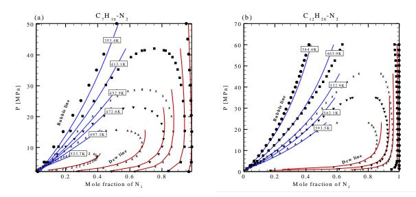
Figure A.1 Phase diagram of hydrocarbon and nitrogen mixture, in which the solid line denotes the results
