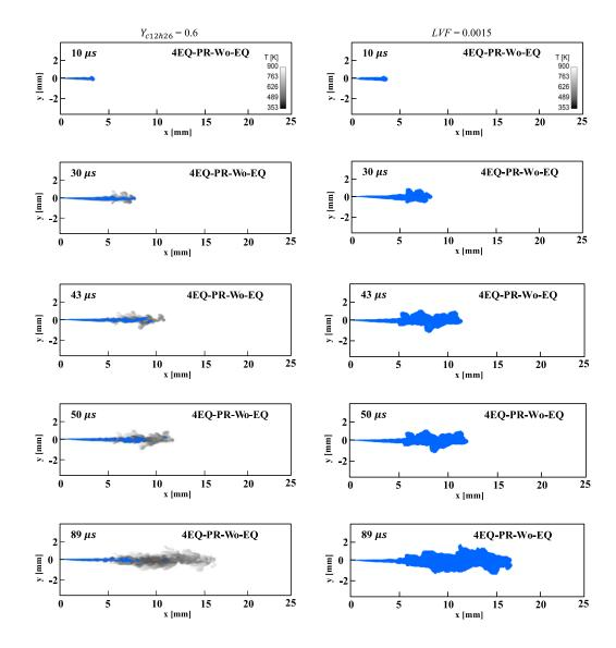
Figure A.3 Illustration of jet evolution from 4EQ-PR-Wo-EQ model at different time instants. The liquid penetration length denoted with blue iso-surface is determined with the mixture mass fraction of  $n-C_{12}H_{26}$ criterion ( $Y_{c12h26} = 0.6$ ) in the left column and the liquid volume fraction criterion (LVF = 0.0015) in the right column. The background contour represents the temperature distribution ranging from 353 K to 900 K.
