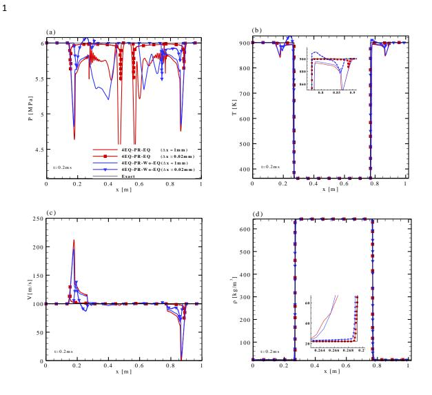
Figure 4 1D advection tube operated with Spray A thermal conditions ( $T_{fuel} = 363 K, P_{amb.} = 6 MPa, T_{amb.} = 900 K$ ). (a, b, c, d) profiles present the evolution of pressure, temperature, velocity and density at 0.2 ms with the two varied mesh sizes of 1mm and 0.2 mm, respectively.
