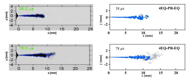
Figure 19 Illustration of early jet evolution for case 2 ( $T_{amb.}$  = 700 K,  $P_{amb.}$  = 4.6 MPa). The liquid 7 8 penetration length marked with blue iso-contour is presented with the criterion of  $LVF = \{0.0015\}$ . The 9 experimental left column is the images snapped directly from **ECN** website (https://ecn.sandia.gov/dbi675/). The right column corresponds to the results of 4EQ-PR-EQ model. The 10 background contour represents the temperature field at the range of 353 K-700 K. 11
