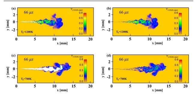
1 Figure 20 Demonstration of the mass fraction of vaporous dodecane  $(Y_{c12h26,vapor})$  for case 1 (Fig.(a, b)) 2 and case 2 (Fig.(c, d)) at the time instant of 66 µs. The two-phase zone is denoted with the iso-surface of 3 TPD equaling 2 as illustrated in the white zone of Fig. (a, c).
