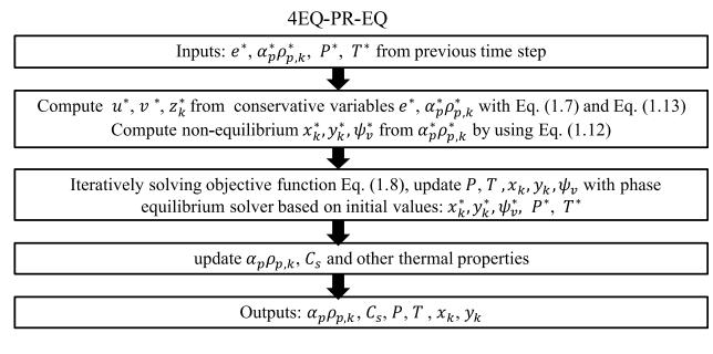
23 Figure 1 Flow chart of 4EQ-PR-EQ model, the inputs denoted by (\*) are the solution from the flow solver.
