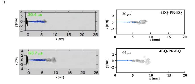
2 Figure 18 Illustration of early jet evolution for case 1 ( $T_{amb.} = 1200$  K,  $P_{amb.} = 8$  MPa). The liquid 3 penetration length marked with blue iso-contour is presented with the criterion of  $LVF = \{0.0015\}$ . The 4 column is the experimental images snapped directly from **ECN** website left 5 (https://ecn.sandia.gov/dbi675/). The right column corresponds to the results of 4EQ-PR-EQ model. The 6 background contour represents the temperature field at the range of 353 K-1200 K.
