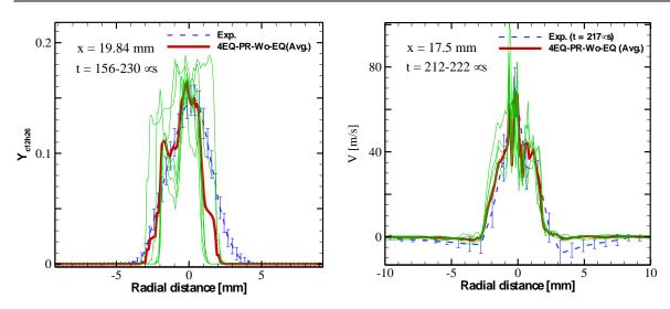
Figure 12 Validations of mixture mass fraction (Left side) and velocity (Right side) with experiments at an axial distance of 19.84 mm and 17.5 mm from the nozzle exit respectively. The instantaneous LES results (green solid line) and the average value (red bold line) are from 4EQ-PR-Wo-EQ model. The experimental data at 217  $\mu$ s (blue dash line) are referred to [55], [57].
