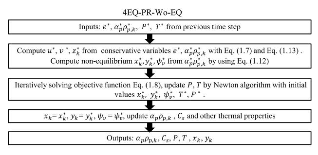
Figure 2 Flow chart of 4EQ-PR-Wo-EQ model, the inputs denoted by (\*) are the solution of the flowsolver.
