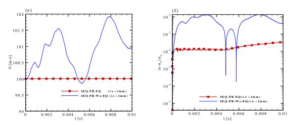
Figure 5 1D advection tube operated with Spray A thermal conditions ( $T_{fuel} = 363 K, P_{amb.} = 6 MPa, T_{amb.} = 900 K$ ). (e, f) profiles illustrate the variation of average velocity and error of total energy in one cycle (10 ms) with the mesh size of 1mm and a CFL value equaling 0.2, respectively.
