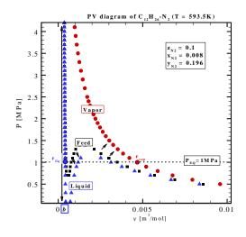
Figure A.2 Schematic of Pv diagram based on the molar fraction feed ( $z_k$ , black square), liquid molar fraction ( $x_k$ , blue triangle). And vapor phase molar fraction ( $y_k$ , red point) at a constant temperature of 593.5 K. The black arrow mimics the phase split process.
