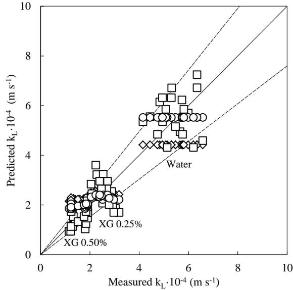
Figure 14: Comparison between different correlations to estimate the oxygen transfer rate. ( $\circ$ ) This work, ( $\square$ ) Kawase et al. 1991, ( $\diamond$ ) Calderbank and Moo-Young 1961, (----)  $\pm 10\%$ , (—) parity line.
