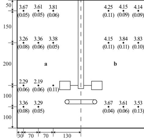
Figure 5: Sauter mean diameter in mm and gas holdup (in brackets) in the large tank. Data were collected for  $N = 8.3 \text{ s}^{-1}$  and for  $U_G = 8 \text{ mm s}^{-1}$  (a) and  $U_G = 20 \text{ mm s}^{-1}$  (b). The probe locations are also indicated.
