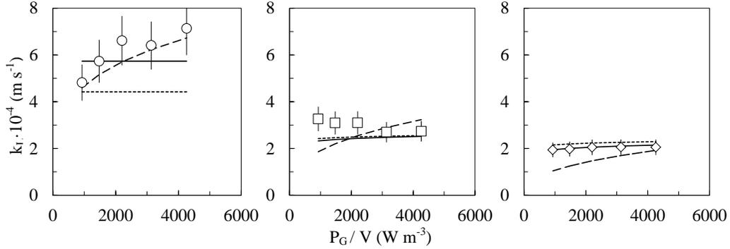
Figure 13: Liquid-side mass transfer coefficient for  $U_G = 8 \text{ mm s}^{-1}$  and predicted values. ( $\circ$ ) water, ( $\square$ ) XG 0.25%, ( $\diamond$ ) XG 0.50%, (—) Equation 11, (---) Kawase et al. 1991, (-----) Calderbank and Moo-Young 1961.
