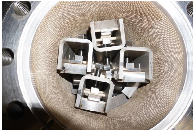
Figure 8 Samples placed in the autoclave with isolating grid to avoid contact between the samples and the internal surface of the reactor
