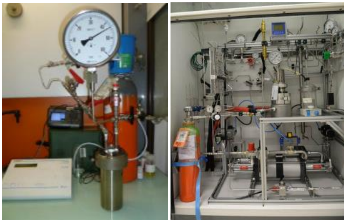
Figure 2: Test devices for pH measurements at pressures up to 45 bara (left) and up to 80 bara (right).
