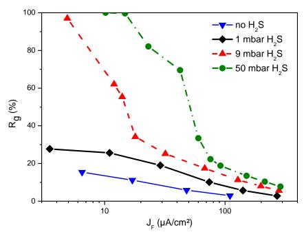
Figure 11 :Evolution of the permeation efficiency ( $R_g = J_{perm}/J_F$ ) with the cathodic current density, measured on 0.5 mm high strength steel membrane exposed to pH 4.5 solutions with varying H<sub>2</sub>S levels, from Plennevaux.<sup>25</sup>
