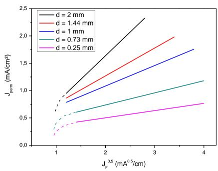
Figure 5: Evolution of the stationary permeation rate with the square root of the cathodic charging current density (1N H<sub>2</sub>SO<sub>4</sub> + 5 mg/L As<sub>2</sub>O<sub>3</sub>), for pure iron membranes of different thickness (data from Dillard <sup>18</sup>).
