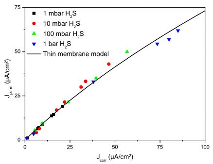
Figure 8: Permeation current vs. corrosion current density for a 0.5 mm thick steel membrane exposed to acid water with dissolved  $H_2S$  (from Duval <sup>8</sup>). Comparison with the predictions of equation (41) (thin membrane model) with  $J_{Fcrit} = 200 \,\mu\text{A/cm}^2$ .
