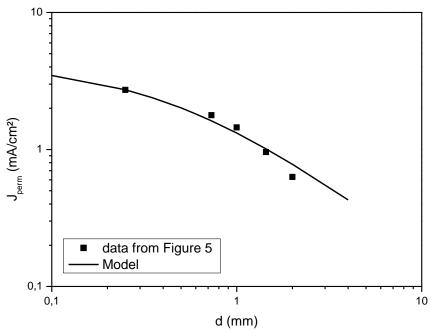
Figure 6: Evolution of the permeation current density with the membrane thickness, from the results of Figure 5 at 3 mA $^{1/2}$ .cm $^{-1}$  (i.e. a cathodic current of 9 mA/cm $^2$ ). Comparison with the model, with  $d_{crit}$ = 0.45 mm and  $v_{Fcrit}$ = 2 mA/cm $^2$ .
