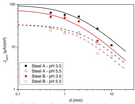
Figure 9: Illustration of the impact of membrane on the steady state permeation flux for different experiments under 100 mbar H<sub>2</sub>S and 900 mbar CO<sub>2</sub> (from Kittel <sup>9</sup>), and comparison with calculated permeation rates (equation [39]).
