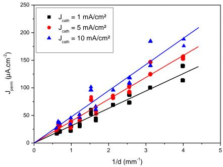
Figure 7: Steady state permeation fluxes through Armco iron membranes of various thickness for respectively -1 (a), -5 (b) and -10 mA/cm² (c) cathodic charging in 1 N H<sub>2</sub>SO<sub>4</sub>, fromAntaño-Lopez <sup>19</sup>.
