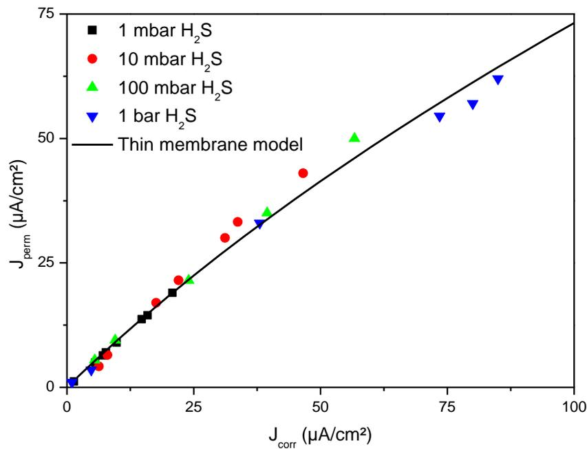
**Figure 8: Permeation current vs. corrosion current density for a 0.5 mm thick steel membrane exposed to acid water with dissolved  $H_2S$  (from Duval<sup>8</sup>). Comparison with the predictions of equation (41) (thin membrane model) with  $J_{Fcrit} = 200 \mu A/cm^2$ .**
