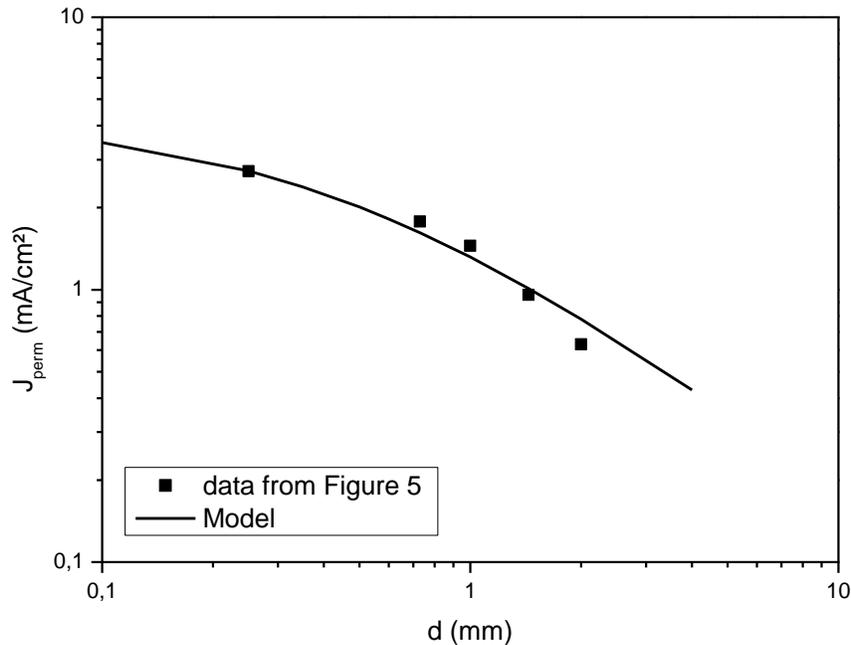
Figure 6: Evolution of the permeation current density with the membrane thickness, from the results of Figure 5 at 3 mA<sup>1/2</sup>.cm<sup>-1</sup> (i.e. a cathodic current of 9 mA/cm<sup>2</sup>). Comparison with the model, with  $d_{crit} = 0.45$  mm and  $v_{Fcrit} = 2$  mA/cm<sup>2</sup>.
