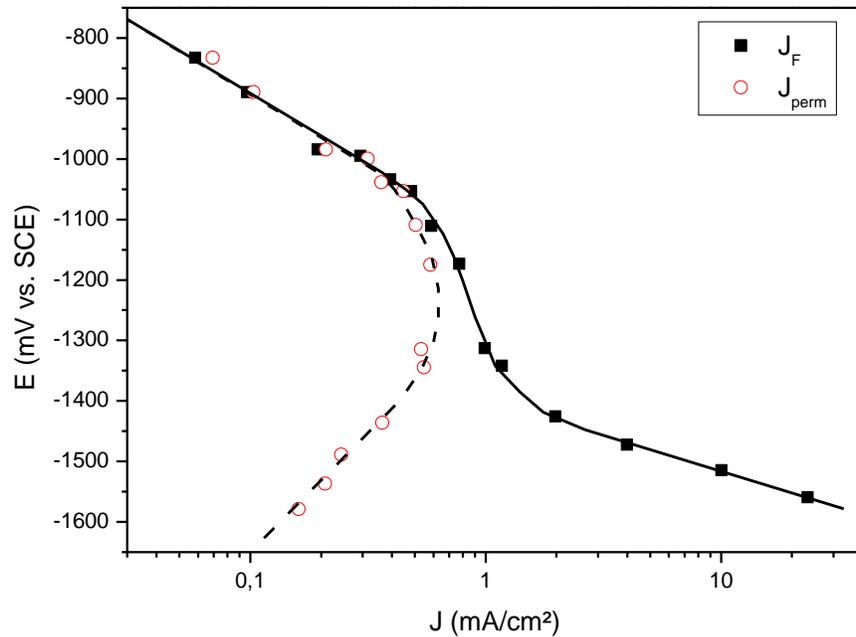
**Figure 10: Comparison between the evolution of the cathodic current density and the permeation current density with the electrode potential, measured on 0.04 mm mild steel membranes exposed to 10 mM NaCl solution with 6.5 mM dissolved H<sub>2</sub>S and at pH 4.35 (data from Le Boucher<sup>22</sup>).**
