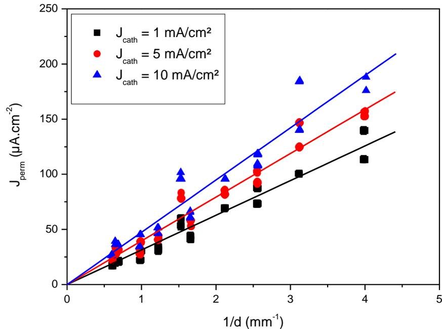
**Figure 7: Steady state permeation fluxes through Armco iron membranes of various thickness for respectively -1 (a), -5 (b) and -10 mA/cm<sup>2</sup> (c) cathodic charging in 1 N H<sub>2</sub>SO<sub>4</sub>, from Antaño-Lopez<sup>19</sup>.**
