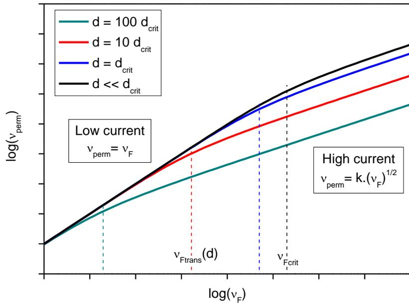
**Figure 2: theoretical evolution of  $v_{perm}$  with  $v_F$  for different values of membrane thickness, corresponding to case 3 above (low surface coverage and low dilute absorbed hydrogen in the metal subsurface).**
