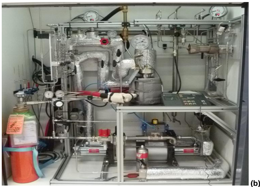
Figure 2: Experimental devices for pH measurements in confined environments at pressure up to 10 bara (a) and up to 100 bara (b)
