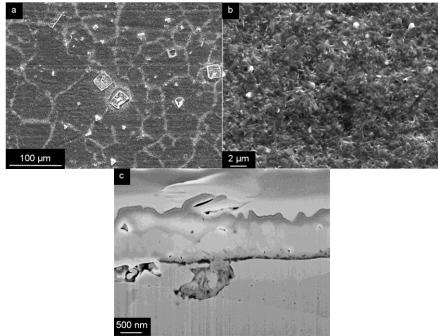
FIGURE 7 SEM micrographies of HR-120 under low oxygen partial pressure at 900°C
