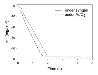
FIGURE 2 TGA curve of a crucible with 50 mg of NaCl under Ar/O<sub>2</sub> and syngas atmosphere at 900°C
