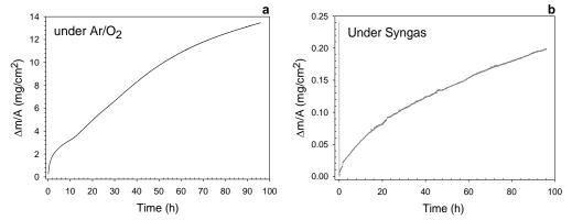
FIGURE 4 TGA of HR-120 with sodium chloride at 900°C under high oxygen partial pressure (a), and under low oxygen partial pressure (b)
