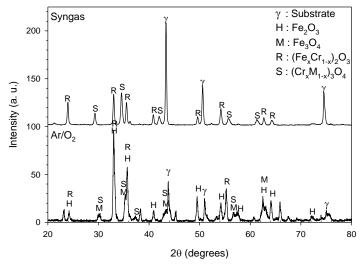
FIGURE 5 XRD of HR-120 after 96 h at 900°C with sodium chloride under high and low oxygen partial pressure
