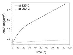
FIGURE 8 Kinetic oxidation of HR-120 under syngas atmosphere in presence of sodium chloride
