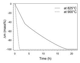
FIGURE 9 Kinetic evaporation of sodium chloride under syngas atmosphere
