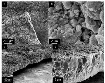
FIGURE 6 SEM micrographies of HR-120 under high oxygen partial pressure at 900°C
