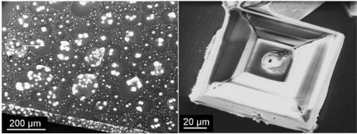
FIGURE 1 SEM surface view of NaCl salt particles after a heating step at 150°C
