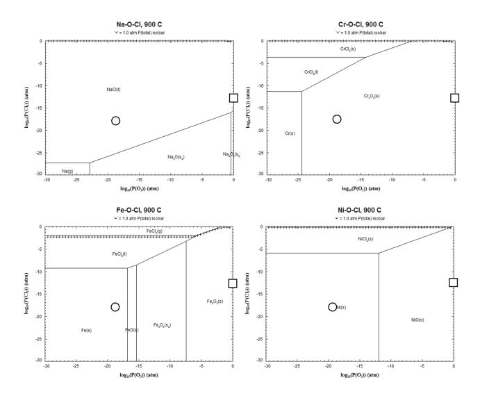
**FIGURE 3** Stability diagrams of Na-O-Cl (**a**), Cr-O-Cl (**b**), Fe-O-Cl (**c**) and Ni-O-Cl (**d**) at 900°C and P=P<sub>atm</sub> Circle: Low oxidising atmosphere; Square: High oxidising atmosphere
