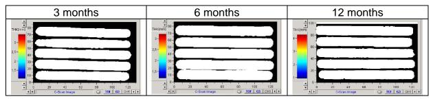
Figure 5: HIC results on a mild sour high strength carbon steel grade tested at pH 5.5 under 1 mbar H<sub>2</sub>S for 3 months to 1 year
