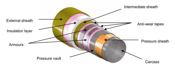
Figure 1: Example of a flexible pipeline structure
