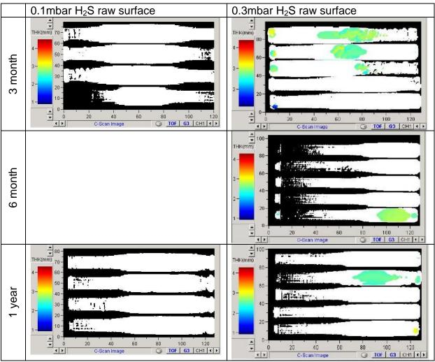
Figure 4: Evolution of HIC extent on sweet steel (A) specimens exposed at ambient temperature and pressure in a 35 g/L NaCl solution saturated with 999.7 mbar  $CO_2$  + 0.3 mbar  $H_2S$  and with 999.9 mbar  $CO_2$  + 0.1 mbar  $H_2S$ .
