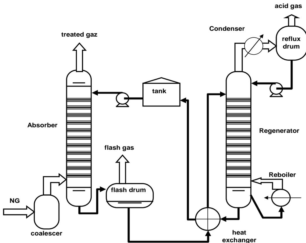
Figure 1: Simplified diagram of an alkanolamine acid gas removal unit
