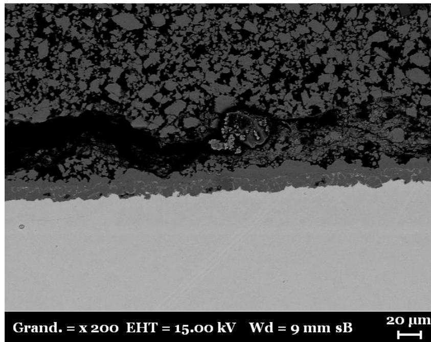
*Figure 2: iron carbonate layer formed at the surface of AISI 1020 coupon after 4 weeks exposure in rich DEA at 110°C.*
