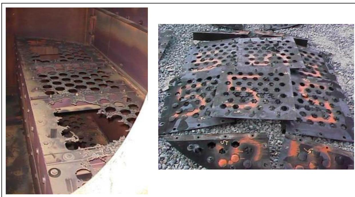
*Figure 2: Examples of uniform corrosion on AISI 410 internals in sweet service amine unit [4].*
