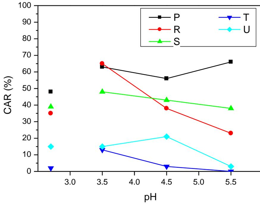
Figure 8: Impact of pH on CAR values for the 2 week exposure under 100mbar H<sub>2</sub>S (points at pH 2.7 corresponds to test in NACE solution, without pH adjustment).
