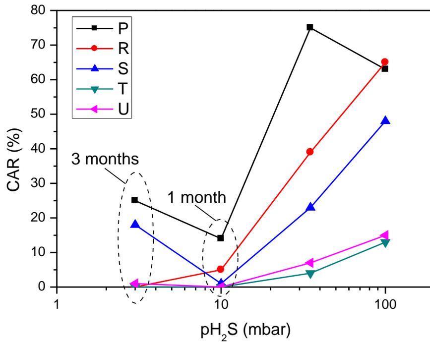
Figure 7: Impact of H<sub>2</sub>S partial pressure on CAR for the experiments at pH 3.5.
