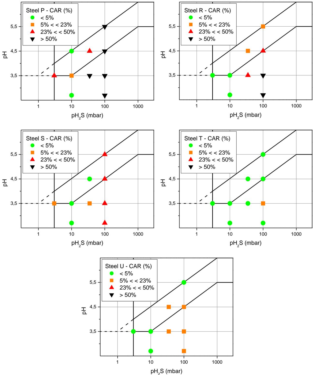
Figure 10: Representation of CAR results in the pH-pH<sub>2</sub>S diagram. Exposure time was 2 weeks for all experiments, except at pH 3.5 – 10mbar (4 weeks) and at pH 3.5 – 3mbar (3 months). EFC 16 solution A was used for all tests, except for tests at pH 2.7, where NACE TM0284-2003 solution A was used.
