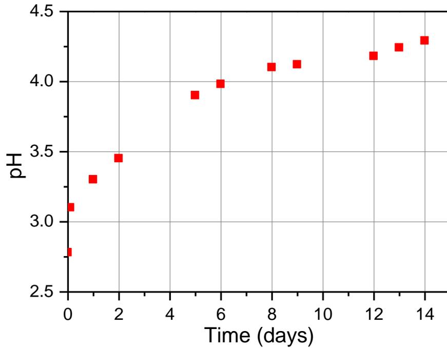
Figure 9: pH evolution during 2 weeks test in NACE TM0284-2003 Solution A under 100mbar H<sub>2</sub>S.
