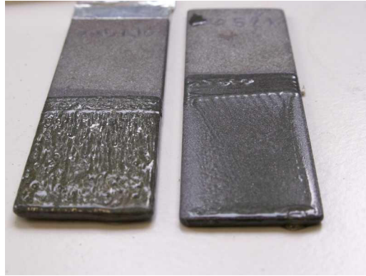
Figure 13 – Films electrodeposited on steel panels during 3 days exposure to a solution of organic film-former agents at 20°C under cathodic polarisation: -1.5 \text{ V}_{/\text{Ag}/\text{AgCl}} (left) ; -0.85 \text{ V}_{/\text{Ag}/\text{AgCl}} (right).
