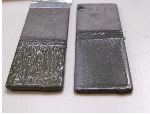
Figure 13 – Films electrodeposited on steel panels during 3 days exposure to a solution of organic film-former agents at 20°C under cathodic polarisation: -1.5 \text{ V}_{/\text{Ag}/\text{AgCl}} (left) ; -0.85 \text{ V}_{/\text{Ag}/\text{AgCl}} (right).
