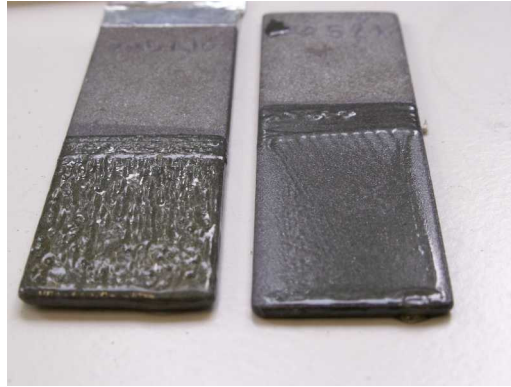
Figure 13 – Films electrodeposited on steel panels during 3 days exposure to a solution of organic film-former agents at 20°C under cathodic polarisation: -1.5 \text{ V}_{/Ag/AgCl} (left) ; -0.85 \text{ V}_{/Ag/AgCl} (right).
