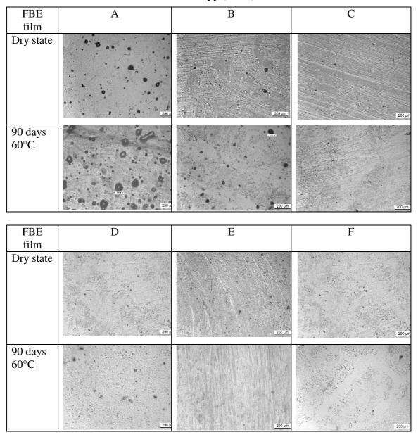
For the second part of the study, two epoxy powders were selected for their differing behaviours in terms of water content and durability while exposed to deionised water at 60°C:
