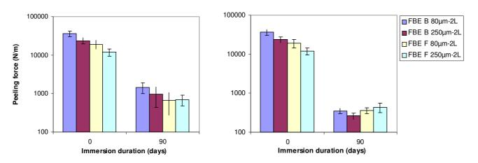
Figure 4 - Peeling force of 2L coatings aged in deionised water at 20°C (left); 60°C (right).
