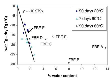
Figure 2 - Delta Tg versus water content for the 6 FBE materials during ageing.
