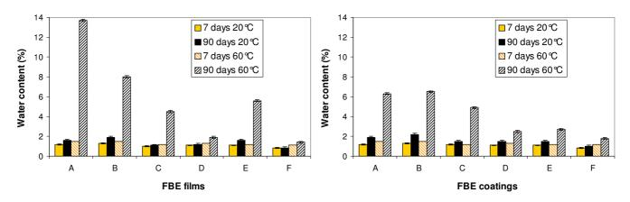
Figure 1 - Water content (wgt. %) measured in FBE films (left) and coatings (right) during ageing in deionised water after 7 days and 90 days at 20°C and 60°C
