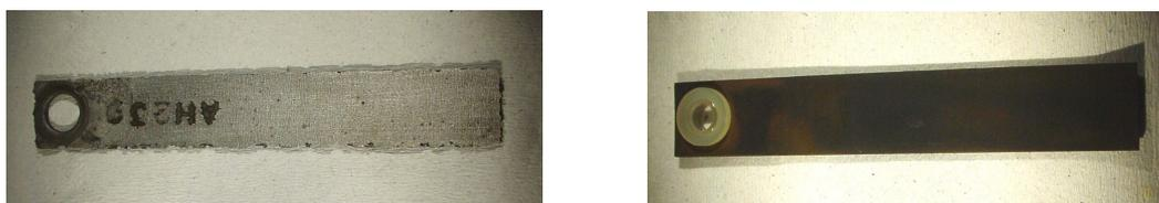
Figure 2: Corrosion coupons removed from the lean amine section at the outlet of the stripper (left) and removed from the CO<sub>2</sub> gas outlet of the stripper.
