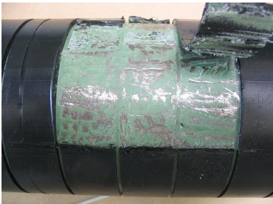
Figure 5 - Peeling of the B-3LPE coating as received
