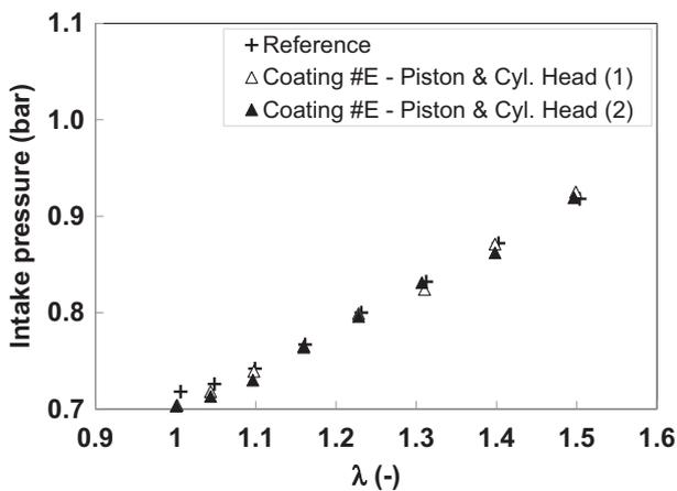
Fig. 11. Intake pressure at 3000 rpm, 7 bar IMEP.
