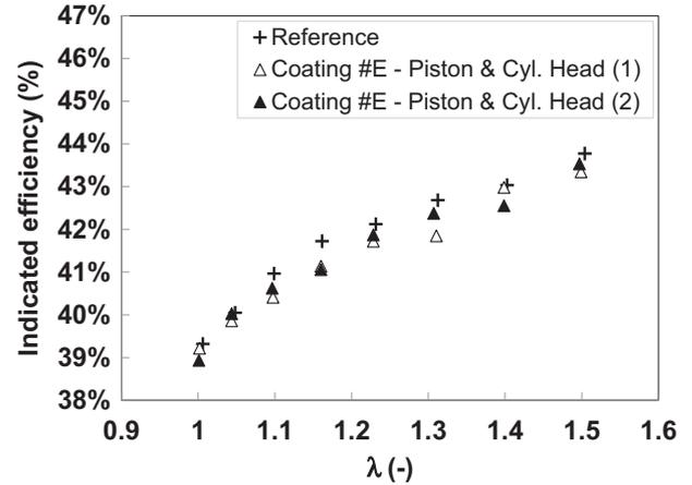
Fig. 13. Indicated efficiency at 3000 rpm, 7 bar IMEP.
