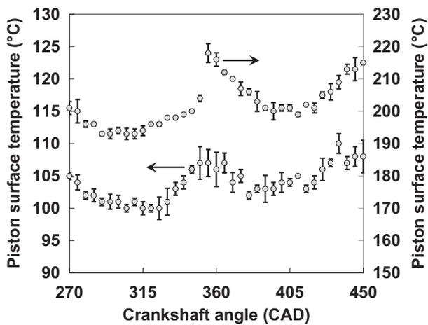
Fig. 4. Piston surface temperatures for uncoated aluminum pistons in motored conditions at 1500 rpm (left axis) and at 2000 rpm, 4 bar IMEP ( $\lambda = 1.21$ , right axis).
