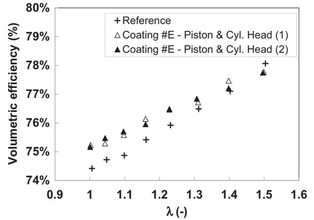
Fig. 12. Volumetric efficiency at 3000 rpm, 7 bar IMEP.
