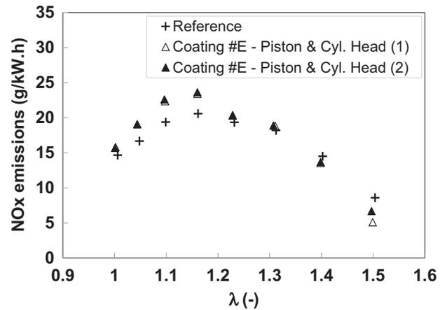
Fig. 15. NOx emissions at 3000 rpm, 7 bar IMEP.
