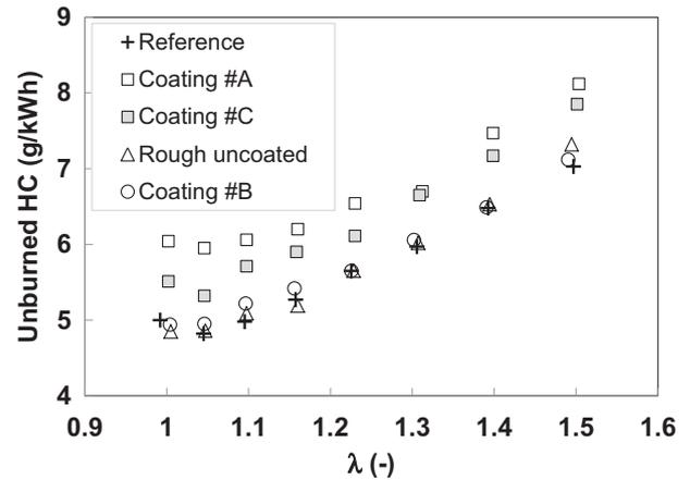
Fig. 8. Unburned hydrocarbon emissions at 3000 rpm, 7 bar IMEP.
