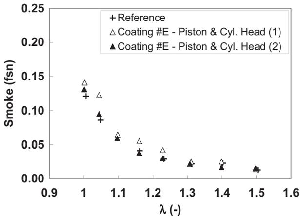
Fig. 10. Smoke emissions at 3000 rpm, 7 bar IMEP.
