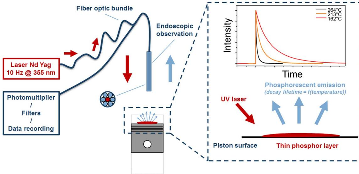
Fig. 1. LIP setup for surface temperature measurement.
