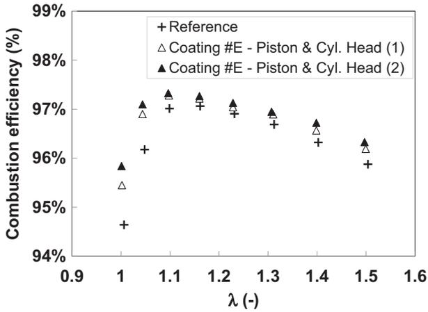
Fig. 9. Combustion efficiency at 3000 rpm, 7 bar IMEP.
