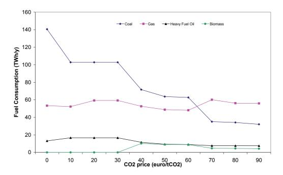
Figure 4: Sensitivity analysis of the fuel consumption with respect to the  $CO_2$  prices for 2020
