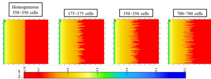
Fig. 2: Comparison of saturation profiles after 0.08 pore volume of water injection when considering homogeneous and porosity/permeability-perturbed models, and three spatial discretizations.
