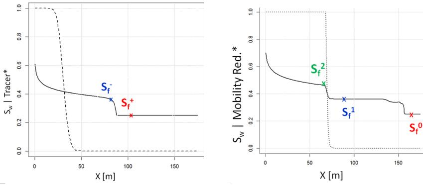
(a) Waterflooding. This saturation profile shows the rarefaction wave and the shock, or saturation front, between the upstream displacing fluid and the downstream fluid-in-place. The dashed line represents a normalized tracer profile or the saturation profile that would correspond to a piston-like displacement.
