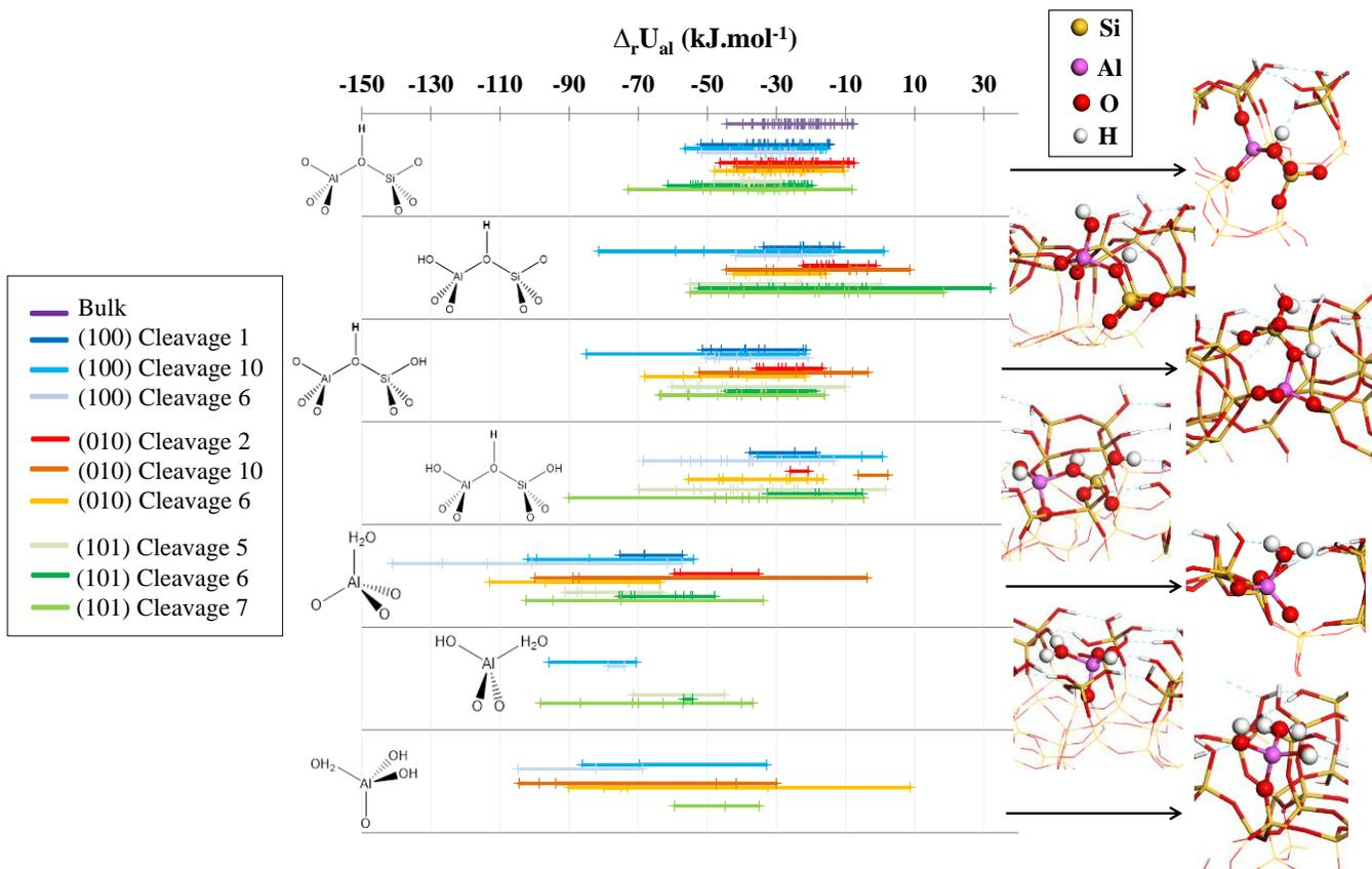
**Figure 5.** Almination energy along the various considered cleavages, and in the bulk of ZSM-5, for the large variety of considered aluminated sites. On the right, the site corresponding to the lowest almination energy for a given kind of site is shown.
