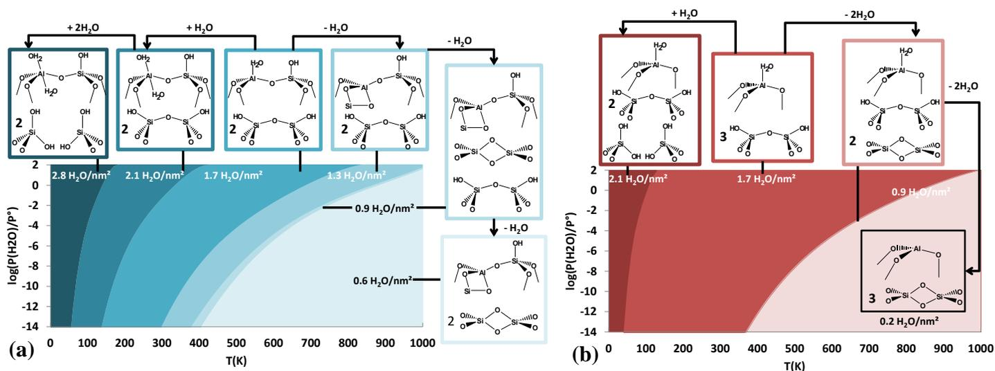
**Figure 6.** Surface hydration thermodynamic diagram for two types of Al-(H<sub>2</sub>O) sites belonging to the Cleavage 1 of (100) surface of ZSM-5. (a) site n°59 and (b) site n°75. The terminology of the surface sites is given in Figure S14.
