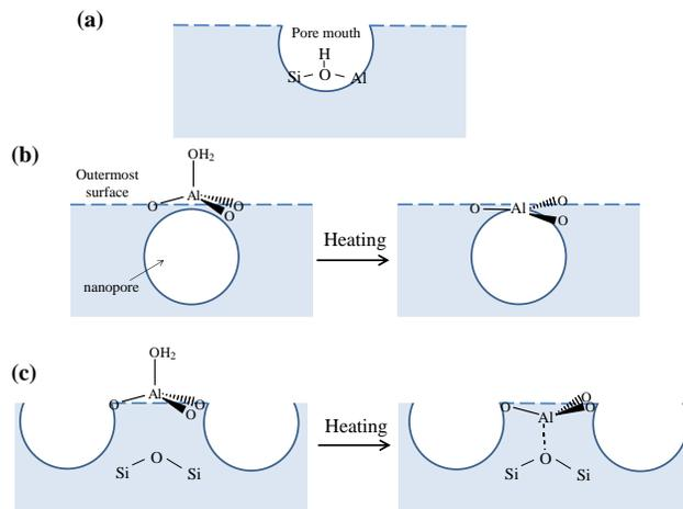
**Figure 7.** Dehydration of Al-(H<sub>2</sub>O)(OH)<sub>n</sub> groups (exemplified in the case of n = 0) depending on the presence of a nanopore (b) or a siloxane bridge (c) below the Al atom, while bridging OH groups at the pore mouth (a) are stable upon dehydration.
