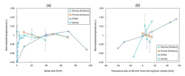
Fig. 23. Comparison of the averaged normalized temperature measured in different ECN facilities: (a) temperature heterogeneity in the spray axis, (b) temperature heterogeneity in the transverse axis at 40 mm from the injector nozzle. *IFPEN* and *Sandia* data from [3].
