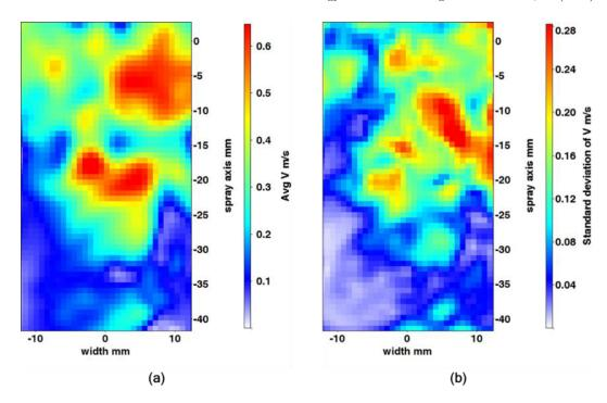
Fig. 12. (a) Average and (b) standard deviation of velocity magnitude at time of injection  $\pm 10$  ms (PPRIME).
