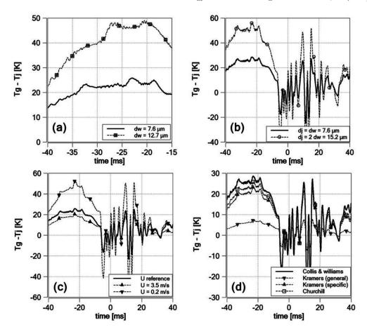
Fig. 17. Main parameters affecting the measured temperature correction: (a) effect of  $d_{\rm w}$ , (b) effect of  $d_{\rm j}/d_{\rm w}$ , (c) effect of the gas velocity  $U(d_{\rm w}=7.6~\mu{\rm m})$ , (d) effect of the Nu correlation ( $d_{\rm w}=7.6~\mu{\rm m}$ ). PPRIME RCM test at spray A target conditions (time axis is referenced to the end of compression).
