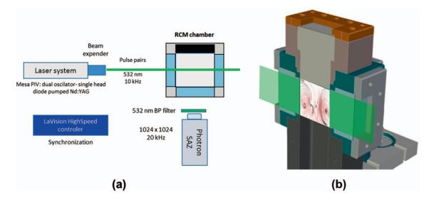
Fig. 8. Schematic of the PIV setup in PPRIME.
