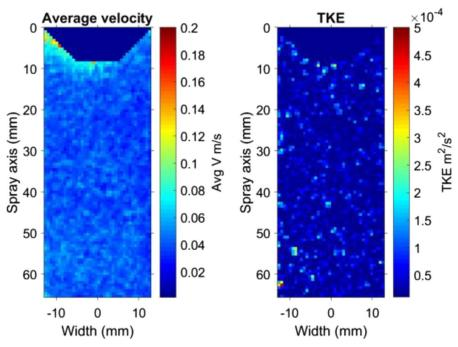
Fig. 14. (a) Average velocity magnitude field and (b) turbulent kinetic energy field at SOI (PRISME).
