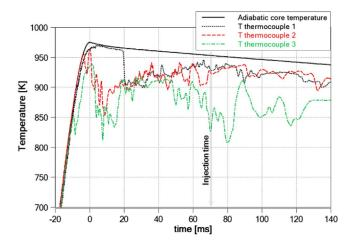
Fig. 19. Illustration of the measured temperature from a single test compared to adiabatic core temperature.
