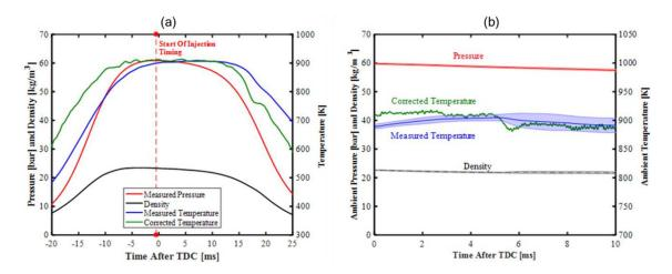
Fig. 21. Illustration of typical temperature profile in *PRISME* (thermocouple 2): (a) example of density, pressure, and temperature profiles around TDC, (b) average temperature profile at 900 K target condition, shaded-error bar represents the standard deviation of 10 measurements.
