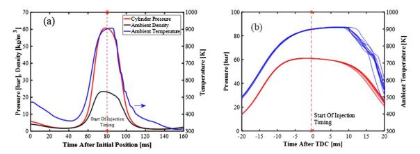
Fig. 6. Thermodynamic condition of NOSE operation: (a) an example of pressure, temperature and density temporal evolution, (b) pressure and temperature evolutions from -20 ms to 20 ms after TDC for 10 repeated tests.
