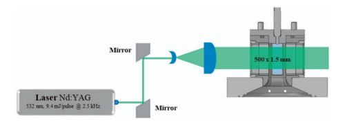
Fig. 9. Schematic of PIV setup in *PRISME*.
