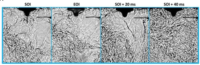
$\textbf{Fig. A1.} \ \, \text{Raw Schlieren images showing thermocouple 4 position and the qualitative density gradients in the RCM chamber at different instants: test condition of Figure 22b.$
