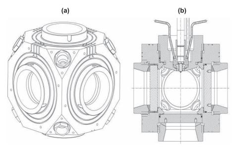
Fig. 1. (a) 3D view and (b) cross section of IFPEN CVP.
