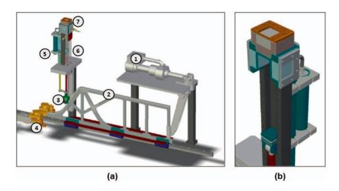
Fig. 2. Schematic of *PPRIME* institute RCM. (a) General view: (1) hydraulic cylinder, (2) cam, (3) guiding wheel, (4) brake system, (5) return pneumatic cylinder, (6) piston/cylinder, (7) combustion chamber. (b) Zoomed section view on the piston cylinder assembly.
