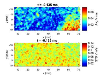
Fig. 10. Average and standard deviation of velocity magnitude at time of injection (*IFPEN* CVP using ensemble average).
