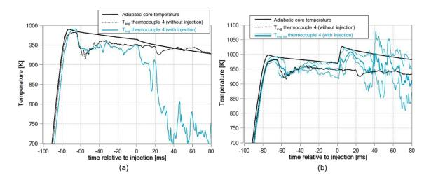
Fig. 22. Temperature measurement in the near nozzle region: (a) at inert conditions, (b) at reactive conditions.
