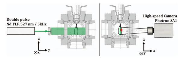
Fig. 7. Schematic of the PIV setup in IFPEN.
