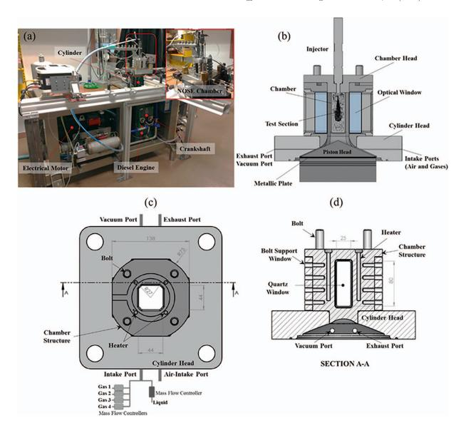
Fig. 4. The NOSE chamber: (a) the overview of real image, (b) the cross-section view in middle plane of chamber, (c) the top-view without chamber head, and (d) the cross-section view A–A without chamber head.
