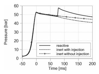
**Fig. 3.** Typical pressure profile of inert and reactive conditions at spray A conditions in *PPRIME*.
