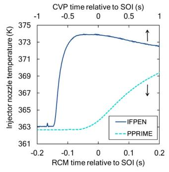
**Fig. 15.** Comparison of the injector nozzle temperature in *IFPEN* CVP and *PPRIME* RCM. The time is referenced to the SOI.
