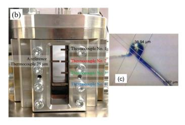
Fig. 20. Location of the temperature measurement in *PRISME*. Four thin-wire thermocouples of 13 μm nominal diameter are used: (a) illustration of measurement positions, (b) picture of thermocouples mounted in the centerline of the NOSE chamber, and (c) picture of the thermocouple junction.
