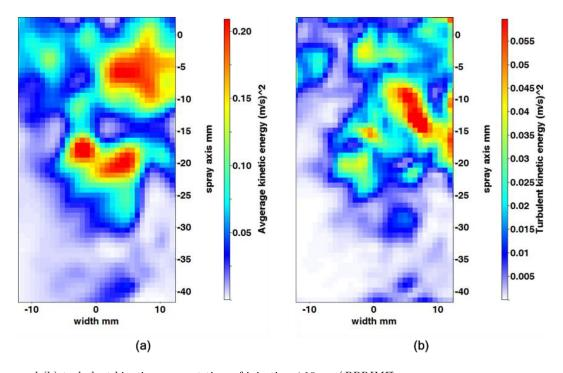
Fig. 13. (a) Average and (b) turbulent kinetic energy at time of injection  $\pm 10$  ms (PPRIME).
