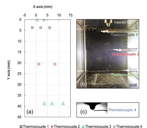
Fig. 18. (a) Illustration of thermocouples positions, (b) picture of thermocouples mounted in the center plane of the *PPRIME* RCM, (c) position of the thermocouple in the near nozzle measurement tests.
