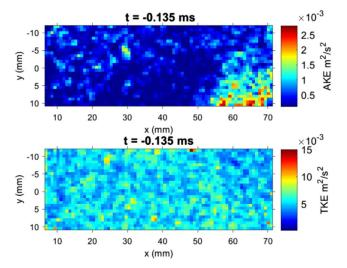
Fig. 11. Average and turbulent kinetic energy at time of injection (*IFPEN* CVP using ensemble average).
