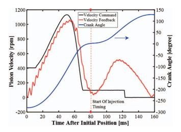
Fig. 5. NOSE operation: comparison of the feedback and command velocities as a function of time referenced to the initial position (280 CAD before TDC).
