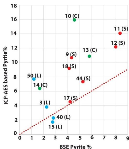
**Figure 4.** Graph illustrating the relationship between inductively coupled plasma-atomic emission spectroscopy (ICP-AES) based pyrite% and scanning electron microscopy (SEM) backscattered electron (BSE) based pyrite%. Red line is plotted along the axis representing an exact match.
