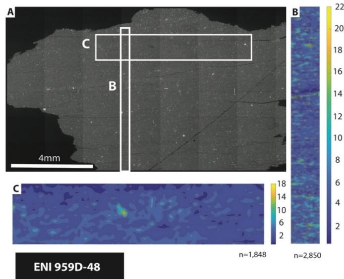
**Figure 8.** (A) Backscattered montage of large area of sample 959D-48. (B,C) are colour contoured maps for organics, from tile sets collected from areas B and C in (A), with 1848 and 2850 tiles, respectively. Individual tile horizontal field of view (HFOV) 60  $\mu\text{m}$ .
