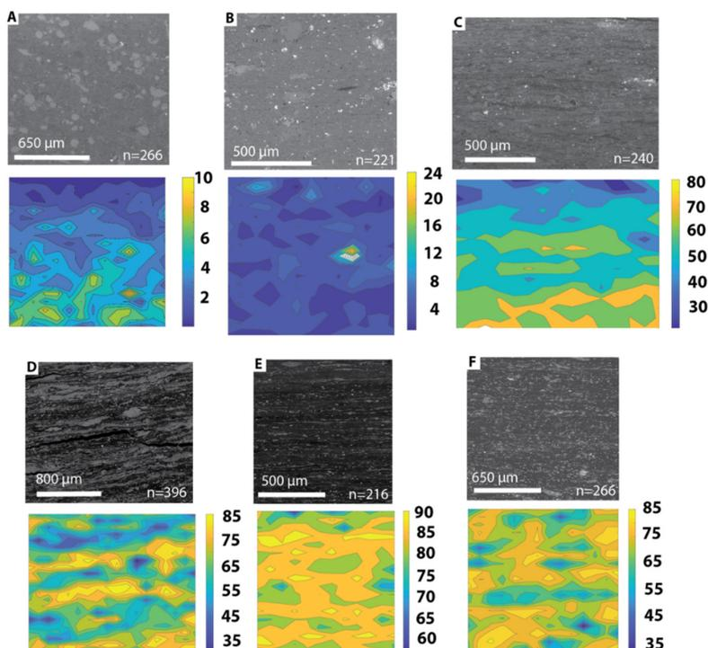
**Figure 6.** (A–F) Pairs of scanning electron microscopy backscattered electron montages and colour contoured organics distribution maps for six Cretaceous mudstones illustrating the distribution of organics. Figure at bottom right = number of tiles in the montage; each tile has a 100  $\mu\text{m}$  horizontal field of view (HFOV). Samples arranged in the same order as Figure 5.
