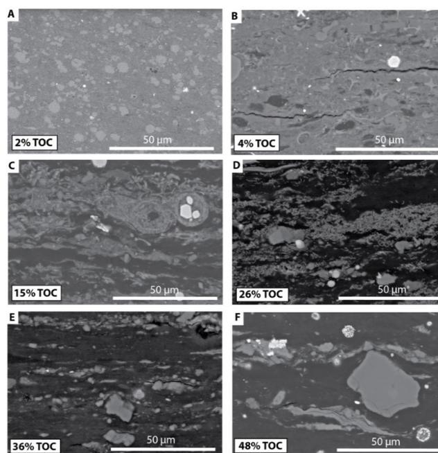
**Figure 5.** Single representative BSE tile images of the six organic samples examined. (A–F) 962D-6, 959D-48, 959D-58, 364-182, 367-20 and 364-205, respectively. Bottom left = recorded TOC from LECO CNS measurements. Note progressive increase in organic content (dark) in BSE images.
