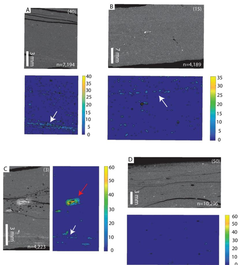
**Figure 2.** (A–D) Pairs of scanning electron microscopy backscattered electron montages and colour contoured pyrite distribution maps for four Jurassic mudstones illustrating sparse pyrite distribution. Figure at top right is sample number, and bottom right is the number of tiles in the montage. Each tile 200  $\mu\text{m}$  horizontal field of view (HFOV). White arrows indicate minor pyrite laminae, and red arrow is a localised concentration.
