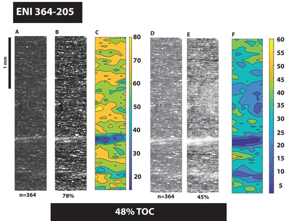
**Figure 9.** (A,D) representative area, BSE montages (364 tiles, each with 100  $\mu\text{m}$  HFOV) of the same area, across thin-section of sample #364-205, with normal contrast (A), and expanded contrast to expand detail at the darker end of the spectrum (D). (B,E) binarized (for organics) of (A,D). (E) with mid-range threshold, binarized and despeckled. (B,E) with 78% and 45% organics, respectively. (C,F) colour contoured map, constructed based on individual tiles from (B,E).
