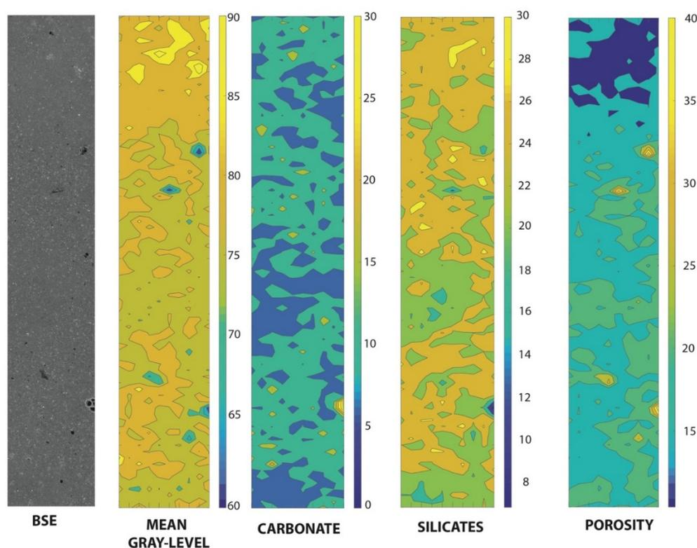
**Figure 11.** Montage through muddy contourite, from the Bay of Cadiz. From left to right: BSE montage, mean grey-level colour contour map, carbonate%, silicates% and porosity% colour contour maps. Montage and colour contoured maps comprise 800 tiles, each with a 300  $\mu\text{m}$  HFOV.
