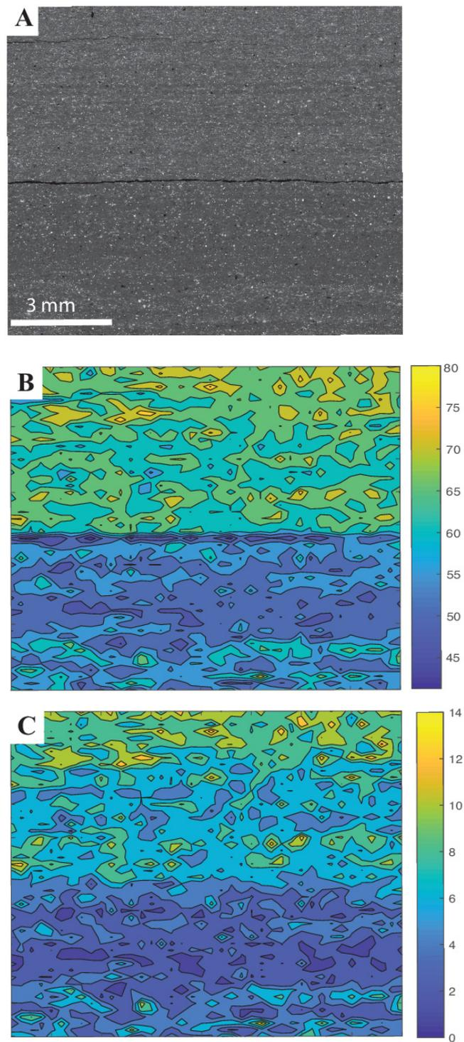
**Figure 10.** Jurassic mudstone sample #9 with (A) BSE montage, (B) mean grey-level (0–256) colour contour map and (C) pyrite percentage colour contour map. Each montage comprises 6557 tiles, with 200  $\mu\text{m}$  HFOV.
