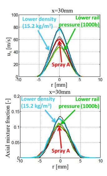
Figure 11 - Velocity (top) and mixture fraction (bottom) radial profiles for different boundary conditions at x=30mm. Solid lines represent the experimental results, black dotted lines the model.
