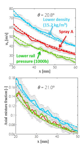
Figure 10 - Velocity (top) and mixture fraction (bottom) axial profiles for different boundary conditions. Solid lines represent the experimental results, dotted lines the model. The grey error bars represent the 95% confidence interval uncertainties
