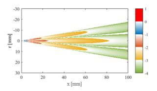
Figure 3 - 2D map of log10( $S_k$ ) based on  $\tau_p$  estimated from the particles characteristics and  $\tau_f$ , extracted from the 1D-spray model based flow acceleration
