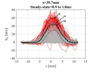
Figure 5 - Top: ensemble averaged radial profiles of the axial velocity, for all the timings between SOI and EOI+2ms. Red profiles are considered to be representative of the steady-state, gray ones are considered transient. Bottom: Same as the top figure, for all the instantaneous radial profiles. The mean  $\mu,$  standard-deviation  $\sigma,$  and uncertainty u are plotted respectively in plain, dotted and dashed black lines.
