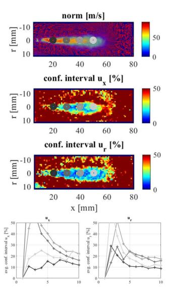
Figure 4 – Top three images: evaluation of the statistical convergence of the ensemble averaged velocity fields, for a delay of  $4\mu$ s, an interrogation window of 16x16 pixels and a timing corresponding to 1.6ms after SOI. Bottom two images: evolution of the confidence interval normalized by the average velocity, for the locations corresponding to the gray circles.
