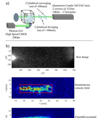
Figure 2 - a) Experimental setup for PIV measurements. b) Example of raw PIV image and related instantaneous velocity field and an ensemble average velocity field. The red rectangle on the instantaneous velocity field indicates the ROI used to estimate peak locking.
