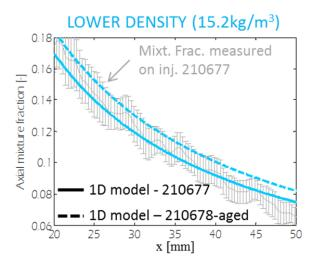
Figure 12 - Comparison of mixture fractions experimental results (in gray) with modeled ones. Solid lines are the estimations from the 1D spray model for injector 210677; dashed lines for injector 210678-aged.
