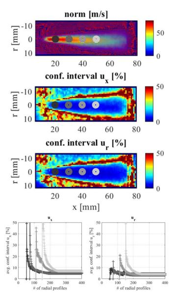
Figure 6 – Top three images: Evaluation of the statistical convergence of the instantaneous velocity fields, for a delay of  $4\mu s$  and an interrogation window of 16x16 pixels after SOI. Bottom two images: evolution of the confidence interval normalized by the average velocity at the locations indicated by the grey cross of the left hand side images.
