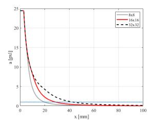
Figure 9 - Axial evolution of |a| for different sizes of interrogation window, and comparison with  $d_{\scriptscriptstyle D}$  (blue dotted line)
