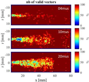
Figure 7 - Influence of the delay  $\Delta t$  between 2 laser pulses on the measured axial velocity for an interrogation window size of 16x16 pixels (top), and on the validity of the computed vectors (bottom three images)
