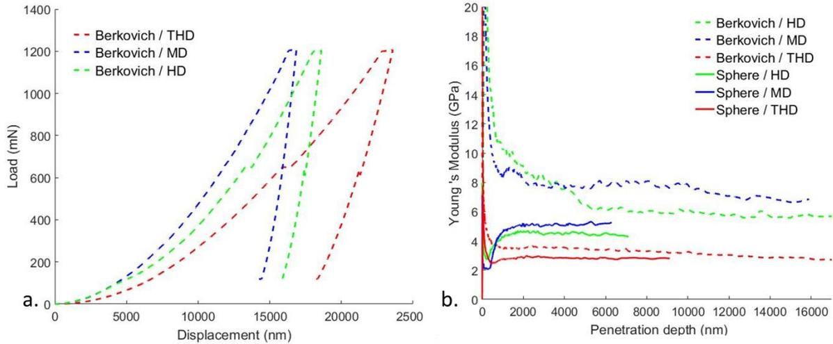
**Figure 8: a) Typical load-displacement measured by Berkovich indenter. b) Young's modulus-penetration depth curves measured of the three-alumina supports by spherical and Berkovich indenter.**
