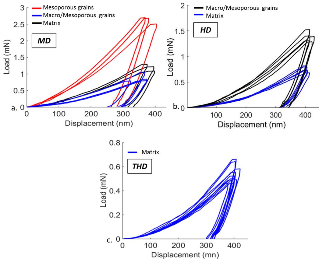
**Figure 10: Load-displacement curves recorded during nano-indentation of constituents of each material: a) matrix (blue), macro- and meso-porous grains (black) and meso-porous grains (red) of the material MD, b) matrix (blue), grains (black) of the material HD, c) matrix of the material THD**
