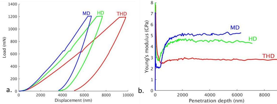
**Figure 6: a) Typical Load-displacement and b) Young's modulus-penetration depth curves of the three alumina supports. The load was maintained at 600 mN during 10 s to allow the change from the "low load" to the "high load" method**
