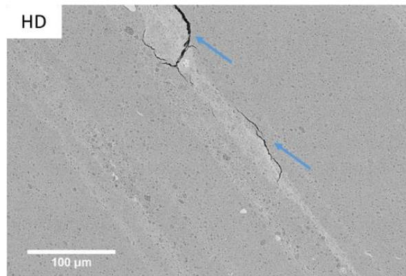
**Figure 14: SEM observation of vertical cuts of alumina support “HD”. The direction of extrusion corresponds to the direction of white lines (densified zones running along the extrudate length). Arrows indicate defects.**
