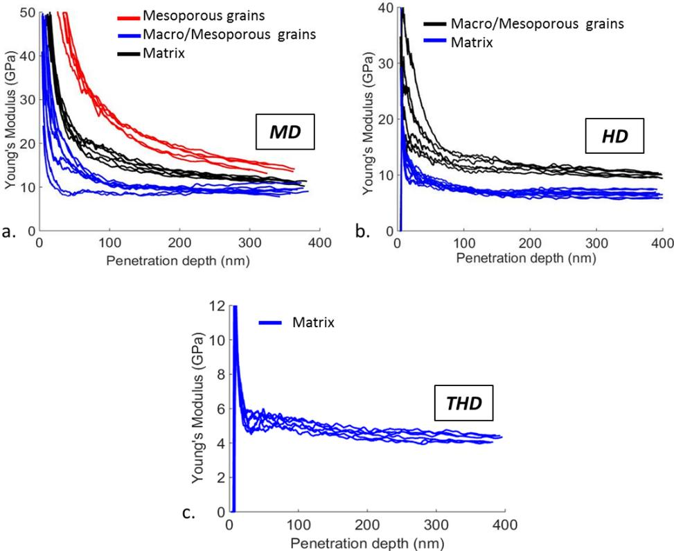
**Figure 11: Indentation Young's modulus versus penetration depth recorded during nano-indentation of constituents of each material: a) matrix (blue), macro- and meso-porous grains (black) and meso-porous grains (red) of the material MD, b) matrix (blue), grains (black) of the material HD, c) matrix of the material THD**
