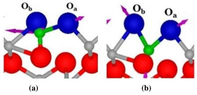
**Fig. 5.** Different vibrational modes of  $CO_2$  molecule; (a) Asymmetric stretching, (b) Symmetric stretching frequency
