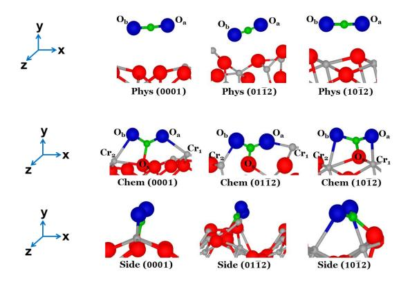
**Fig. 3.** Different optimized adsorption geometries of  $Cr_2O_3$  (0001), (0112) and (1012) surface; The topmost figure represents the physisorbed structure, the middle figure represents chemisorbed species with (x-y plane) view and the figure below represents the side view (y-z plane) of the adsorbed configurations. O atoms of  $CO_2$ , C atoms, surface O atoms and Cr atoms are respectively shown in blue, green, red and dark gray.
