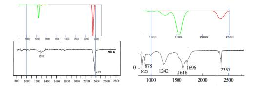
**Fig. 6.** Calculated (above) and experimental (below) [12] IR spectrum of  $CO_2$  on (a) the (0001) versus  $Cr_2O_3$  (0001)/Cr(110) and (b) the (0112) facet versus polycrystalline. The green resonances correspond to the stretching modes of the chemisorbed  $CO_2$  and the red one of the physisorbed  $CO_2$ .Energy in cm<sup>-1</sup>.
