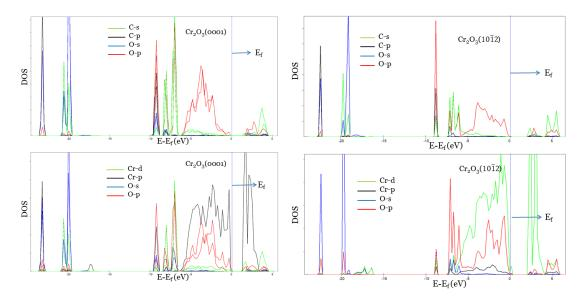
**Fig. 8.** PDOS plots for  $Cr_2O_3$  (0001) and (1012) surfaces. All plots are aligned at the Fermi level.
