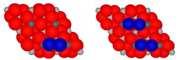
**Fig. 4.**  $CO_2$  coverage  $\Theta$  on (0001)  $Cr_2O_3$  surface calculated per surface-Cr atom (indicated in dark grey): left 25%; right 50%.
