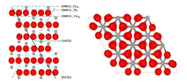
**Fig. 1.** Left: Three different facets (0001), (01 $\overline{1}2$ ), and (10 $\overline{1}2$ ) of chromium oxide surface; (right) top view of 2 × 2 cell (0001) Cr<sub>2</sub>O<sub>3</sub>.
