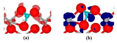
**Fig. 7.** Charge density difference (CDD) plot for (0001)  $Cr_2O_3$  surface (a) positive (in red) and (b) negative for the chemisorbed configuration (in blue). The isosurfaces were plotted at  $\pm 0.06 \text{ e/ } \text{\AA}^3$ .
