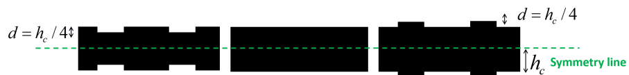
Figure 16: Reduction and increase of the planar-walls channel section by the respective introduction of obstacles and cavities. Middle : planar-wall channel, left: obstacles, right: cavities.
