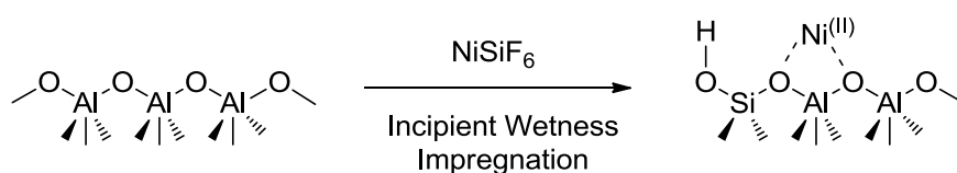
Scheme 7. Expected effect of \text{Al}_2\text{O}_3 impregnation with \text{NiSiF}_6 to create a nickel-aluminosilicate pocket
