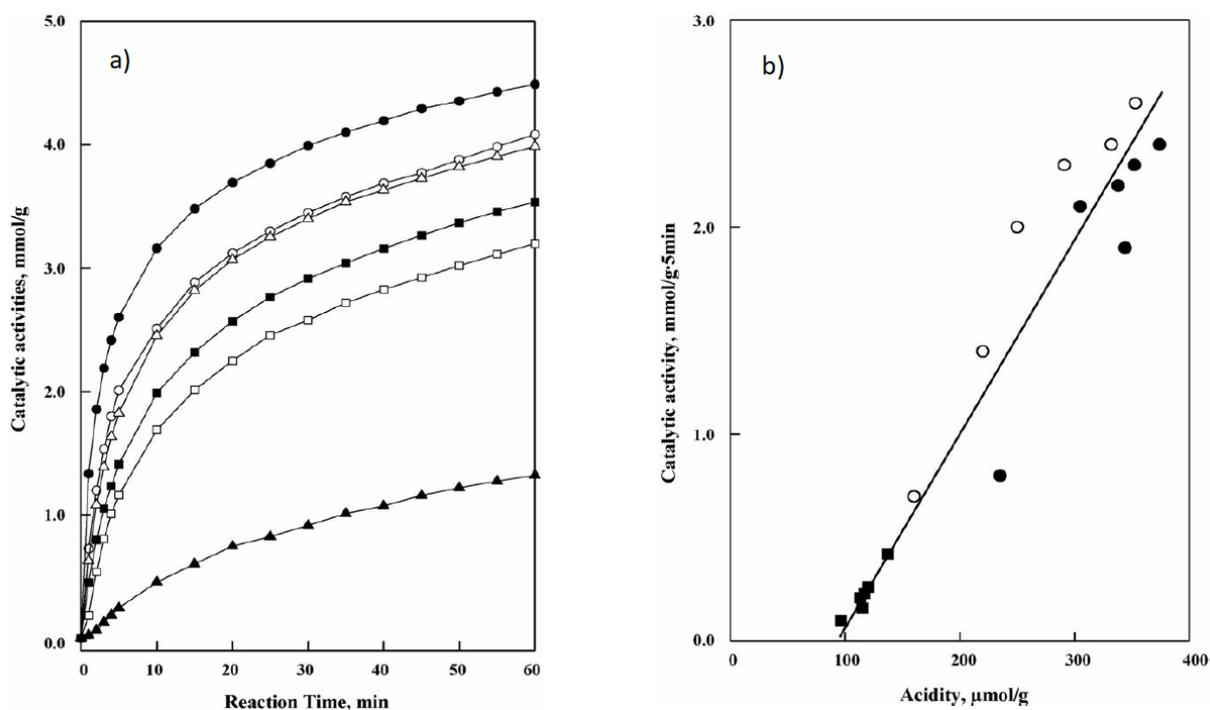
**Figure 39.** a) Catalytic activities of (■) 15-NiSO<sub>4</sub>/82-SiO<sub>2</sub>-Al<sub>2</sub>O<sub>3</sub>; (●) 15-NiSO<sub>4</sub>/66-SiO<sub>2</sub>-Al<sub>2</sub>O<sub>3</sub>; (▲) 20-NiSO<sub>4</sub>/SiO<sub>2</sub> against reaction time and b) Correlation between catalytic activity for ethylene
