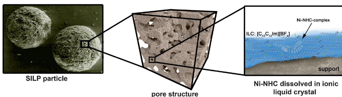
**Figure 38.** Schematic representation of a SILP material composed of ionic liquid crystal  $[\text{C}_{12}\text{C}_{12}\text{Im}][\text{BF}_4]$  with a Ni–NHC complex dissolved therein (reproduced with permission from ref 184. Copyright 2012 The Royal Society of Chemistry).
