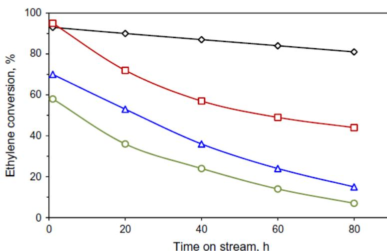
**Figure 44.** Activity profile of (◇) Ni-AlSBA-15 outperforming (□) Ni-MCM-41, (Δ) Ni-SiO<sub>2</sub>-Al<sub>2</sub>O<sub>3</sub> and (○) Ni-Y. (Reproduced with permission from ref 334. Copyright 2015 Elsevier)
