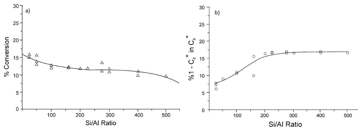
**Figure 40.** a) Ethene conversion and b) 1-Hexene selectivity as a function of Si/Al ratio of the support. T = 100 °C, P = 1.5 MPa, MHSV = 4 h<sup>-1</sup>, and time-on-stream = 280 min. (Reproduced with permission from ref 281. Copyright 2003 Elsevier)
