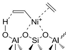
**Figure 52.** DFT-computed intermediate proposed in nickel active site generation in a SSZ-24 zeolite framework<sup>26</sup>
