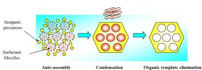
Scheme 6. Synthesis scheme for MCM-41 mesoporous materials
