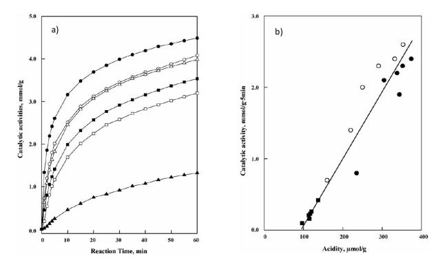
**Figure 39.** a) Catalytic activities of ( $\blacksquare$ ) 15-NiSO<sub>4</sub>/82-SiO<sub>2</sub>-Al<sub>2</sub>O<sub>3</sub>; ( $\bullet$ ) 15-NiSO<sub>4</sub>/66-SiO<sub>2</sub>-Al<sub>2</sub>O<sub>3</sub>; ( $\blacktriangle$ ) 20-NiSO<sub>4</sub>/SiO<sub>2</sub> against reaction time and b) Correlationship between catalytic activity for ethylene
