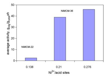
**Figure 42.** Effect of the Ni<sup>2+</sup>/acid sites ratio on the catalytic activity of NiMCM-22 and -36 after 30 minutes (150°C, 40 bar) (Reproduced with permission from ref 311. Copyright 2008 Elsevier)
