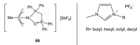
Figure 33. Weakly-coordinating ILs for the biphasic ethylene oligomerization using cationic Nicomplexes
