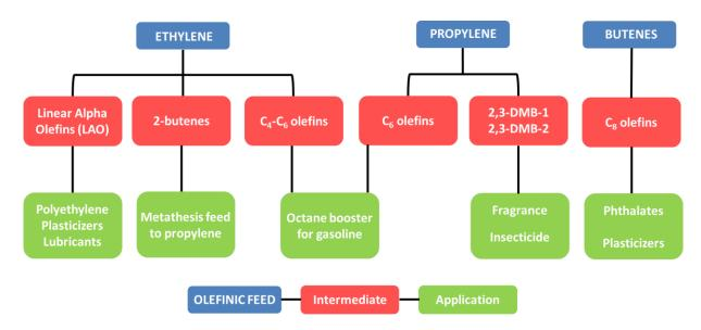
Figure 1. Oligomerization of light olefins to fuels and petrochemical intermediates and their applications
