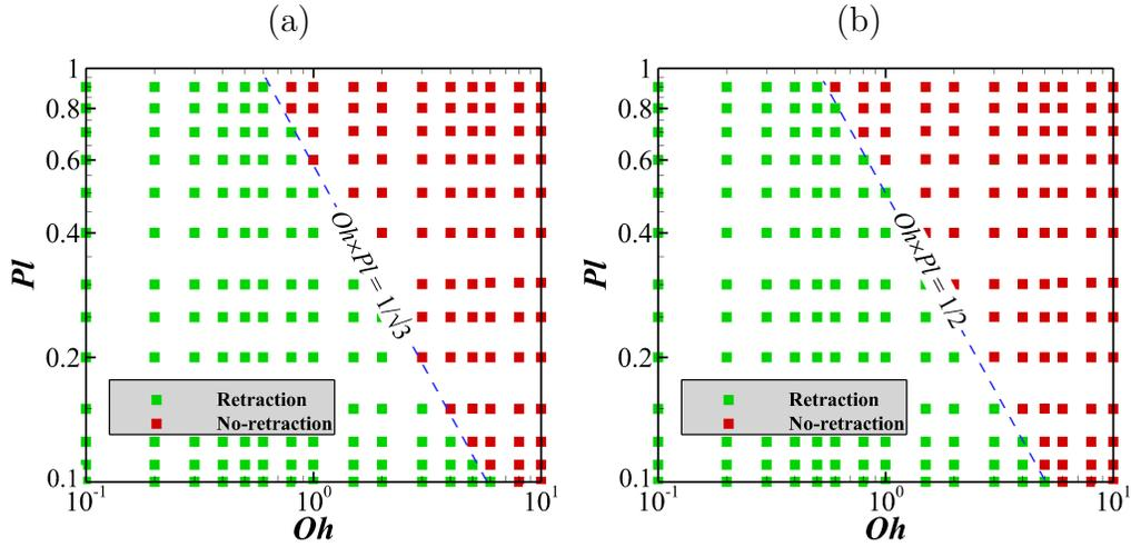
Figure 4. A regime map showing the retraction and no-retraction points in the  $Oh - Pl$  plane for (a) axisymmetric drops and (b) two-dimensional sheets. The red squares represent the points where the drop retraction is resisted by the yield stress of the viscoplastic material and the green squares represent the points where the viscoplastic drops/sheets retract overcoming the yield stress of the material. [Initial aspect ratio is 10 in all the numerical simulations considered here.](#)
