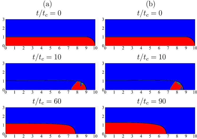
Figure 6. The yielded (blue) and unyielded (red) regions within the viscoplastic slender drops for (a)  $Oh = 2.0$ ,  $Pl = 0.25$  and (b)  $Oh = 3.0$ ,  $Pl = 0.15$  at different time instants. The interface profile at each time instant is shown by the black line.
