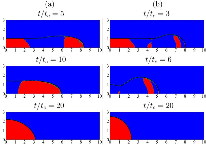
Figure 8. The yielded (blue) and unyielded (red) regions within the viscoplastic slender drops for (a)  $Oh = 0.4$ ,  $Pl = 0.9$  and (b)  $Oh = 0.1$ ,  $Pl = 0.9$  at different time instants. The interface profile at each time instant is shown by the black line.
