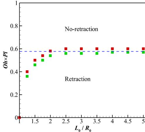
Figure 5. Numerical results showing the retraction and no-retraction regimes of an axisymmetric drop as a function of the initial aspect ratio  $L_0/R_0$ . The red squares represent the points where the drop retraction is resisted by the yield stress and the green squares represent the points where the viscoplastic drops undergo retraction. The dotted line is the theoretical prediction (11).
