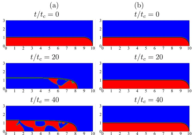
Figure 3. The yielded (blue) and unyielded (red) regions within the viscoplastic liquid sheet for  $Oh = 2.0$  and two different values of plastic number: (a)  $Pl = 0.2$  and (b)  $Pl = 0.3$ . The plots are shown at a dimensionless time interval of  $\Delta t/t_c = 20$ . The interface profile at different time instants is shown by the black line.
