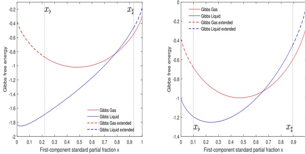
Figure 7: Extended Gibbs energy functions  $g_L$  (blue) and  $g_G$  (red) for Peng-Robinson's law by the indirect method, with  $\varepsilon = 0.001$ . Left panel:  $(A^I, B^I) = (0.322, 0.053)$  and  $(A^{II}, B^{II}) = (0.33, 0.03)$ . Right panel:  $(A^I, B^I) = (0.275, 0.045)$  and  $(A^{II}, B^{II}) = (0.35, 0.04)$ .
