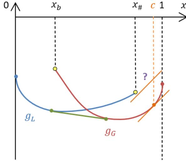
Figure 6: Typical situation where the fraction in the absent phase cannot be computed.
