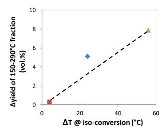
Figure 9: Mapping of hybrid vs. individual catalysts according to the variation in the temperature at iso-conversion and variation in the yield of 150-290°C fraction for the hydrocracking of light VGO (data from Table II in [96]). Catalysts: NiMoS/USY (▲), NiMoS/BEA (
