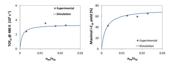
**Figure 4:** Experimental and simulation results for n-hexadecane hydroconversion: a) turnover frequency per protonic site at 480 K and b) maximal feed isomer yield as function  $n_{Pt}/n_{Al}$  ratio for mixtures of 75%Pt/H-USY with 25% of Pt/H-BEA. Adapted from [67] by permission of The Royal Society of Chemistry.
