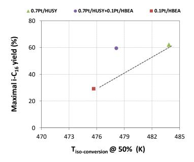
**Figure 5:** Mapping of hybrid vs. individual catalysts according to the temperature at 50% feed conversion and maximal feed isomer yield. Adapted from [67] by permission of The Royal Society of Chemistry.
