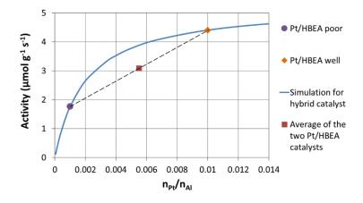
Figure 6: Simulation of catalytic activity for *n*-hexadecane hydroconversion at 480 K as function of  $n_{Pt}/n_{Al}$  over hybrid catalysts consisting of two Pt/HBEA catalysts, in a 50:50 (wt./wt.) mixture. Reproduced from [70].
