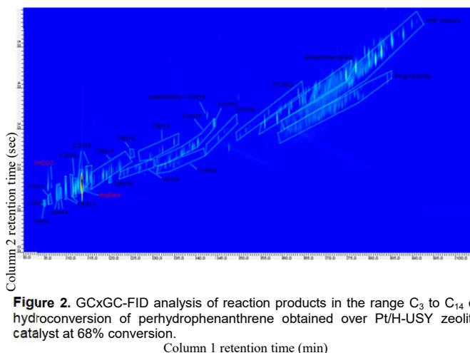
**Figure 2.** GCxGC-FID analysis of reaction products in the range C<sub>3</sub> to C<sub>14</sub> of hydroconversion of perhydrophenanthrene obtained over Pt/H-USY zeolite catalyst at 68% conversion.
