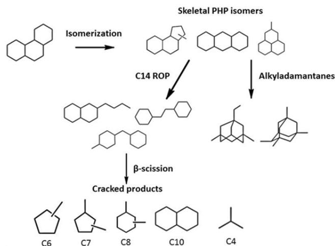
**Figure 14.** General reaction pathway for hydrocracking of perhydrophenanthrene over bifunctional Pt/H-USY zeolite catalyst.
