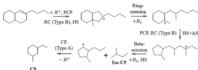
**Figure 20.** Suggested hydrocracking pathways leading to C<sub>9</sub> naphthenes and C<sub>5</sub> isoalkanes. RC: ring-contraction, HS: hydride shift, AS: alkyl-shift, CE: cycle expansion.
