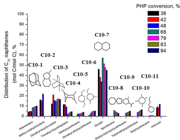
**Figure 13.** Distribution of C<sub>10</sub> naphthenes resulting from hydrocracking of PHP over Pt/H-USY zeolite catalyst at different conversions.
