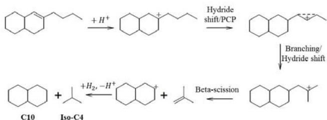
**Figure 18.** Suggested hydrocracking pathway to  $C_{10}$  naphthenes and isobutane of ring-opening product originated from hydroconversion of skeletal perhydrophenanthrene isomers (**R6**) over Pt/H-USY zeolite catalyst.
