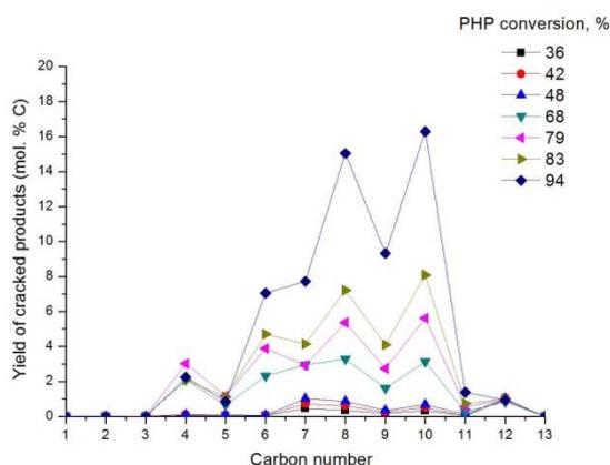
**Figure 10.** Yield of cracked products according to the number of carbon atoms in the molecules at different levels of PHP conversion over Pt/H-USY zeolite catalyst.
