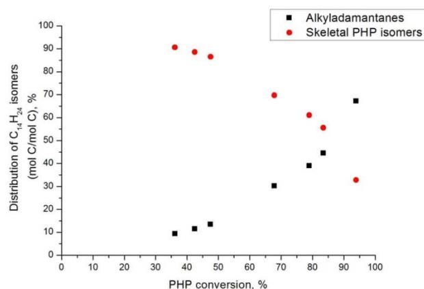
**Figure 6.** Distribution of C<sub>14</sub>H<sub>24</sub> reaction products of PHP conversion over Pt/H-USY zeolite catalyst against PHP conversion.
