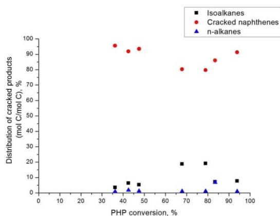
**Figure 11.** Distribution of naphthenes, isoalkanes and n-alkanes in the cracked products based on C-atom content against PHP conversion over bifunctional Pt/H-USY zeolite catalyst.
