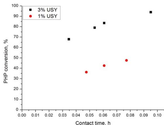
**Figure 4.** Evolution of PHP conversion with contact time on Pt/H-USY catalyst extrudates with 1 wt.% and 3 wt.% zeolite in alumina binder.
