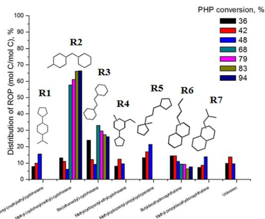
**Figure 9.** Distribution of ring-opening products (ROP) at different PHP conversions over Pt/H-USY zeolite catalyst.
