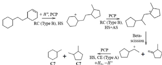
**Figure 17.** Suggested hydrocracking pathway of ring-opening products originating from hydroconversion of skeletal perhydrophenanthrene isomers (**R3**) over Pt/H-USY zeolite catalyst, leading to  $C_7$  naphthenes. RC: ring-contraction, HS: hydride shift, AS: alkyl-shift, CE: cycle expansion.
