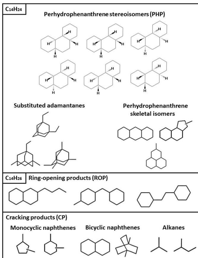
**Figure 3.** Molecule families and typical examples of reaction products of perhydropheanthrene stereoisomers hydroisomerization and hydrocracking over Pt/H-USY zeolite catalyst.
