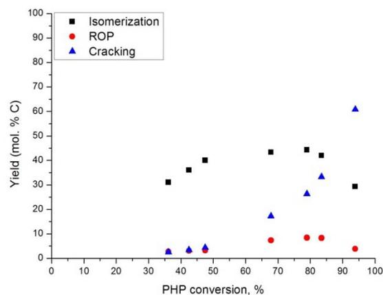
**Figure 5.** Yield of skeletal isomerization, ring-opening and cracked products against perhydropheanthrene conversion over Pt/H-USY zeolite catalyst.
