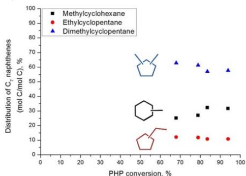
**Figure 12.** Distribution of C<sub>7</sub> naphthenes resulting from hydrocracking of PHP over Pt/H-USY zeolite catalyst.
