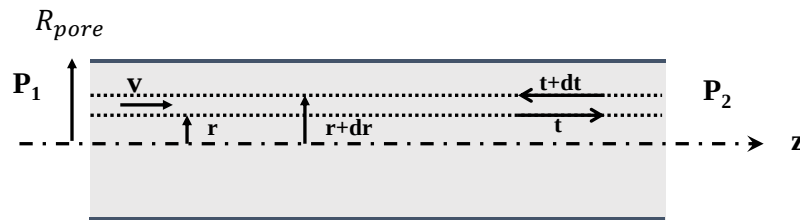
Figure A. 2 - Control volume for a flow within a cylindrical tube of radius R [51]
