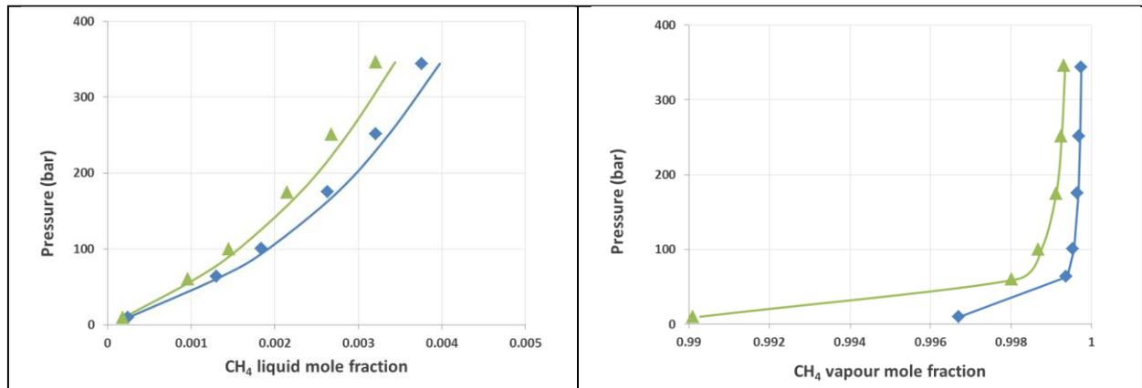
**Figure 8. Pressure-composition diagram of the CH<sub>4</sub>+H<sub>2</sub>O system (left: bubble curves; right: dew curves). Symbols: experimental data [53]. Solid lines: this model. Diamonds: 25 °C. Triangles: 40 °C.**
