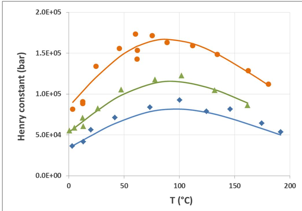
Figure 6. Henry constant of methane in salted water. Symbols: experimental data [50]. Solid lines: this model. Triangles:  $m_{NaCl} = 0.8 \text{ mol/kg}_{H_2O}$ . Circles:  $m_{NaCl} = 1.9 \text{ mol/kg}_{H_2O}$ . Squares:  $m_{NaCl} = 3 \text{ mol/kg}_{H_2O}$ .
