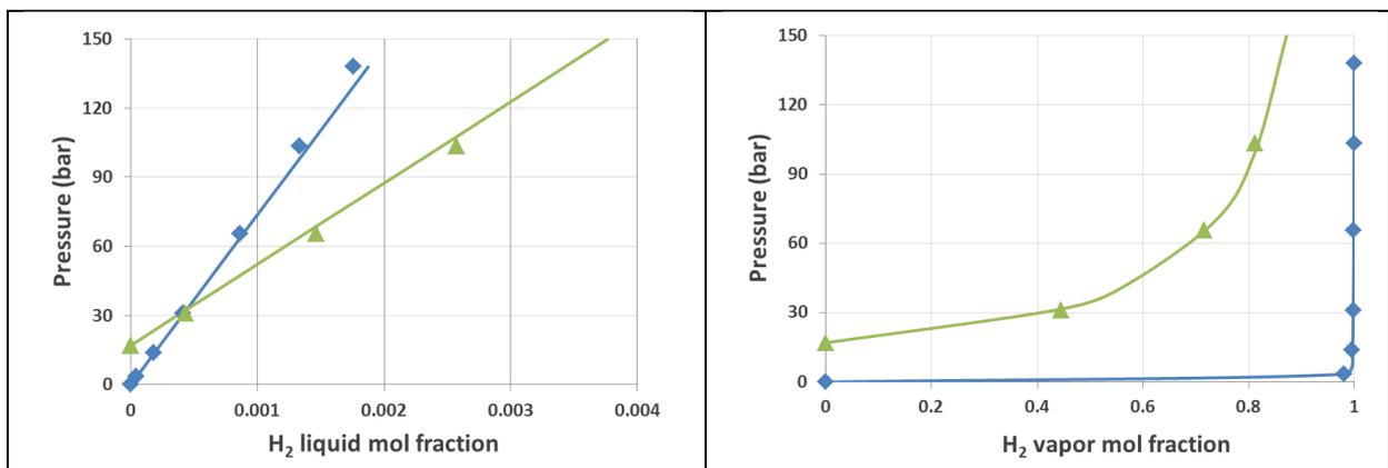
**Figure 7. Pressure-composition diagram of the H<sub>2</sub>+H<sub>2</sub>O system (left: bubble curves; right: dew curves). Symbols: experimental data [52]. Solid lines: this model. Diamonds: 37.8 °C. Triangles: 204.5 °C.**
