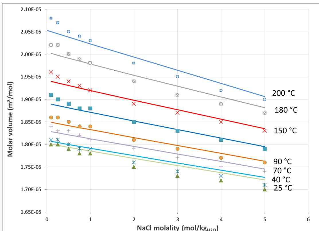
**Figure 3. Liquid molar volumes of aqueous NaCl solutions. Symbols: experimental data [46]. Solid lines: this model.**
