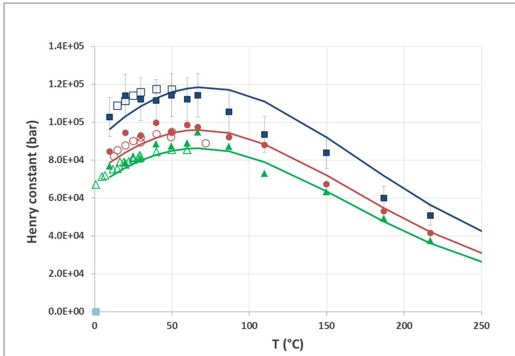
**Figure 5. Henry constant of hydrogen in salted water. Open symbols: experimental data [48,49]. Filled symbols: data from molecular simulation [26]. Solid lines: this model. Triangles:  $m_{NaCl} = 0.5$  mol/kg<sub>H2O</sub>. Circles:  $m_{NaCl} = 1$  mol/kg<sub>H2O</sub>. Squares:  $m_{NaCl} = 2$  mol/kg<sub>H2O</sub>.**
