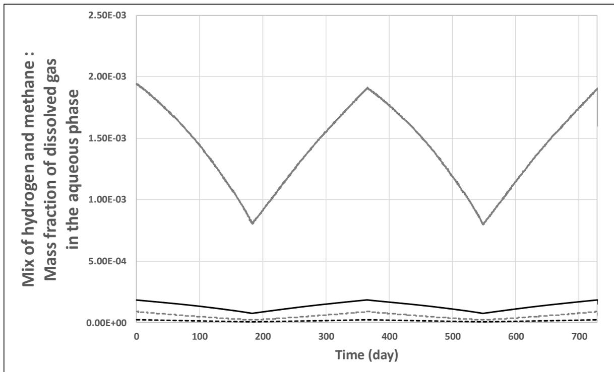
**Figure 11: Mass fraction of dissolved methane (solid line) and dissolved hydrogen (dotted line) in the liquid phase for a mix storage considering brine (black color) or pure water (grey color) as the residual fluid after debrining.**
