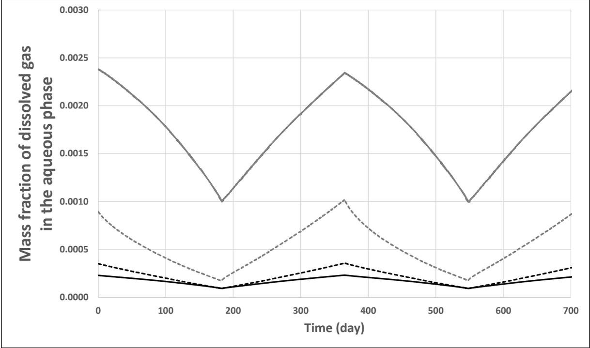
Figure 10: Mass fraction of dissolved methane in the liquid phase for methane storage (solid line) and dissolved hydrogen for hydrogen storage (dotted line) considering brine (black color) or pure water (grey color) as the residual fluid after debrining.
