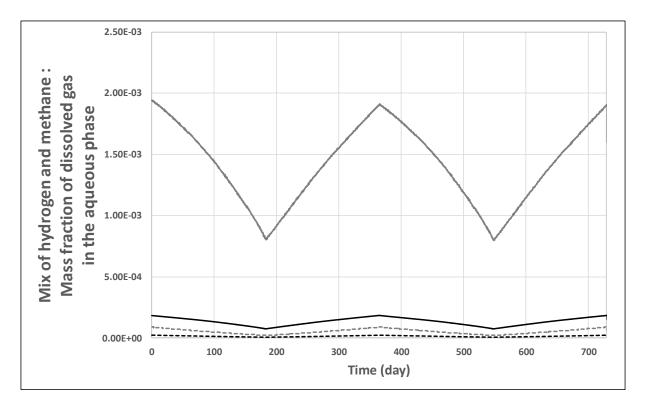
Figure 11: Mass fraction of dissolved methane (solid line) and dissolved hydrogen (dotted line) in the liquid phase for a mix storage considering brine (black color) or pure water (grey color) as the residual fluid after debrining.
