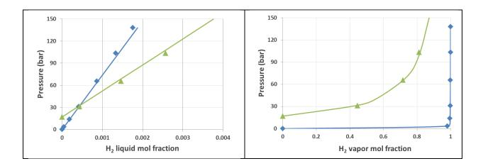
Figure 7. Pressure-composition diagram of the H<sub>2</sub>+H<sub>2</sub>O system (left: bubble curves; right: dew curves). Symbols: experimental data [52]. Solid lines: this model. Diamonds: 37.8 °C. Triangles: 204.5 °C.
