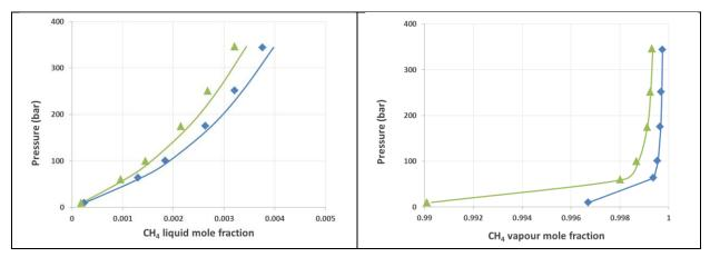
Figure 8. Pressure-composition diagram of the  $CH_4+H_2O$  system (left: bubble curves; right: dew curves). Symbols: experimental data [53]. Solid lines: this model. Diamonds: 25 °C. Triangles: 40 °C.
