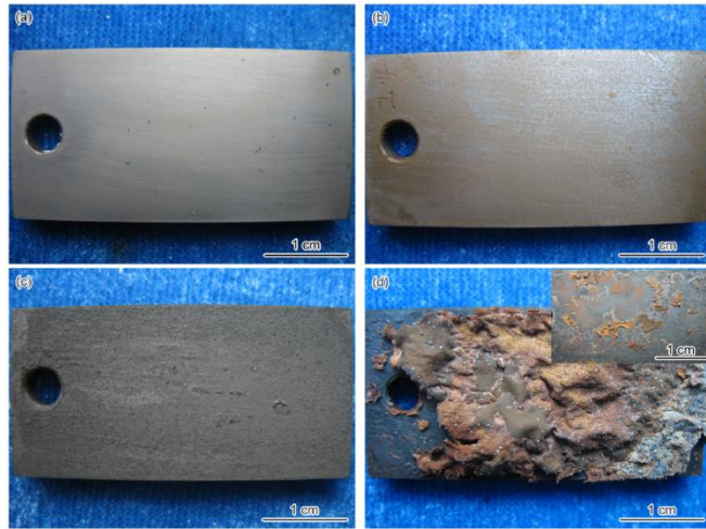
Figure 6 Photographs of corrosion product layer developed at 50°C CO 2 , 10 MPa, O 2 : 2000 ppmv, H 2 S: 2000 ppmv. (a) CO 2 ; (b) CO 2 + O 2 ; (c) CO 2 + H 2 S and (d) CO 2 + O 2 + H 2 S [77].
